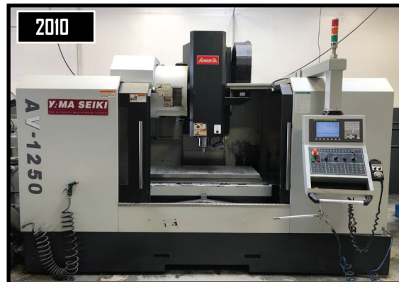
2010 YAMA SEIKI AWEA AV-1250 CNC VMC, W/ 10,000 RPM, CAT 40, 24 ATC, FANUC Oi-MD CONTROL, (XYZ) 49.2" X 24.4" X 24.4", S/N 1250-10006.
