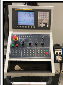
2010 YAMA SEIKI AWEA AV-1250 CNC VMC, W/ 10,000 RPM, CAT 40, 24 ATC, FANUC Oi-MD CONTROL, (XYZ) 49.2" X 24.4" X 24.4", S/N 1250-10006.
