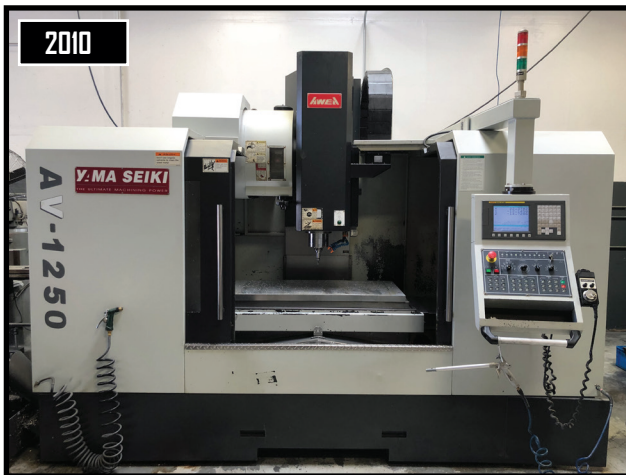
2010 YAMA SEIKI AWEA AV-1250 CNC VMC, W/ 10,000 RPM, CAT 40, 24 ATC, FANUC Oi-MD CONTROL, (XYZ) 49.2" X 24.4" X 24.4", S/N 1250-10006.
