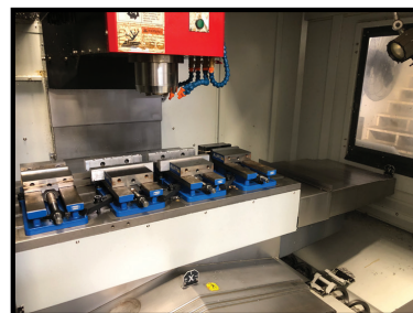
2015 YAMA SEIKI AWEA AV-1060 CNC VMC, W/ 15,000 RPM, CAT 40, 30 ATC, FANUC Oi-MF CONTROL, 2455 RUN TIME, 3 AXIS, (XYZ) 41.7" X 23.6" X 23.6", S/N 1060-15059.
