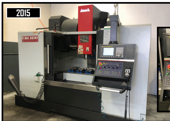
2015 YAMA SEIKI AWEA AV-1060 CNC VMC, W/ 15,000 RPM, CAT 40, 30 ATC, FANUC Oi-MF CONTROL, 2455 RUN TIME, 3 AXIS, (XYZ) 41.7" X 23.6" X 23.6", S/N 1060-15059.
