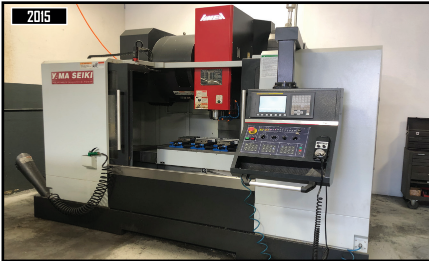
2015 YAMA SEIKI AWEA AV-1060 CNC VMC, W/ 15,000 RPM, CAT 40, 30 ATC, FANUC Oi-MF CONTROL, 2455 RUN TIME, 3 AXIS, (XYZ) 41.7" X 23.6" X 23.6", S/N 1060-15059.
