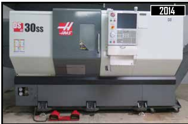
Haas DS30SS Twin Spindle Live Turret CNC Turning Center w/ Tool Presetter, 12-Station Live Turret, 4500 RPM, 6000 Live RPM, Rigid Tapping
