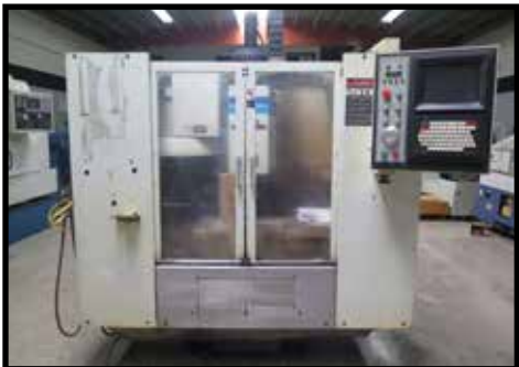
Fadal VMC40 CNC VMC w/ Fadal CNC88 Controls, 21-Station ATC
