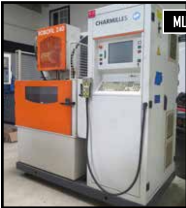
2001 Charmilles Robofil 240 CNC Wire EDM Machine w/ Charmilles Controls.
