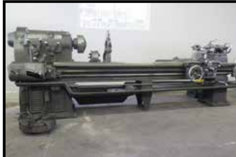
Monarch 16W 16" x 102" Geared Head Lathe w/ 12-487 RPM, Taper Attachment
