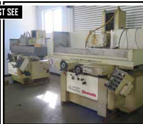
Okamoto ACC-16-32DX 16" x 32" and ACC-12-24DX 12" x 24" Auto Surface Grinders
