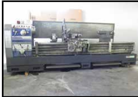
Victor 29120T 29" x 120" Geared Head Gap Bed Lathe w/ 1200 RPM, Inch/mm Threading, 4" Thru Spindle
