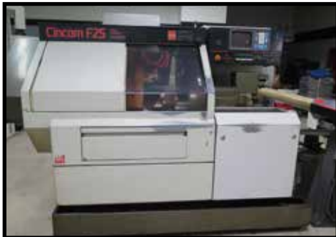
Citizen Cincom F25 1" Cap. Twin Turret CNC Screw Machine w/ Fanuc Controls, Twin 5-Station Turrets
