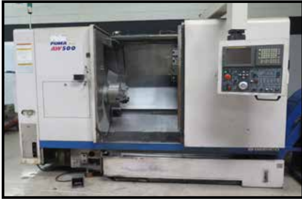
2000 Daewoo PUMA AW500 CNC Turning Center w/ Fanuc 18i-T Controls, 12-Station Turret, 3000 RPM
