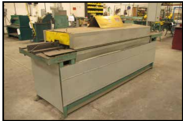
Lockformer HVAC Rollformer
