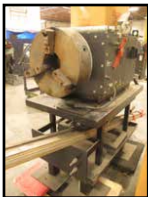
CYPRESS PIPE PLASMA CUTTING LINE, BUG-O-SYSTEM W/ 16" 3 JAW CHUCK, HYPER THERM POWER MAX PLASMA.
