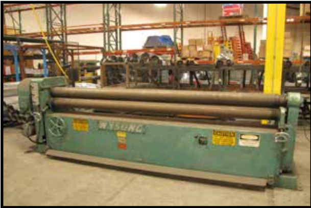
WYSONG 10FT INITIAL PLATE ROLLS, 6" ROLLS, MECHANICAL.
