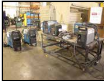
PARTIAL VIEW OF MILLER WELDERS AND HYERTHERM PLASMA CUTTERS.
