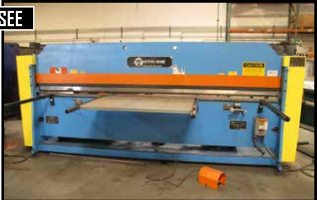
ROTO DIE MODEL 10 HYDRAULIC BRAKE, WITH MANUAL BACK GAGE
