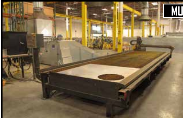
ESAB PIECEMAKER 2 CNC PLASMA TABLE, 5FT X 20FT, HYPER THERM PLASMA 1250, ATAS VISION LE-5 CONTROL.
