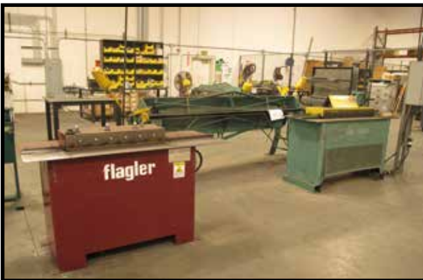
PARTIAL VIEW OF FLAGLER, LOCKFORMER AND OTHER ROLLFORMERS HVAC.
