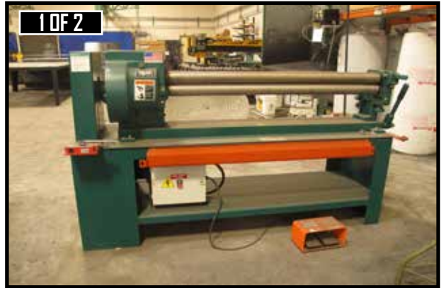
(1 OF 2) TENNSMITH SR48P, 48" X 16GA INITIAL PINCH PLATE ROLLS.
