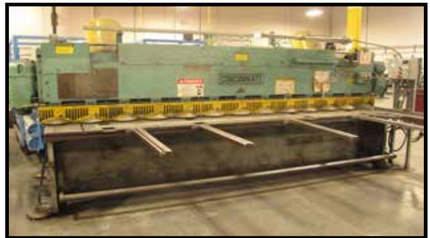
CINCINNATI 1412, 12FT X 3/16 MECHANICAL POWER SHEAR, W/ POWER BACK GAGE, SQUARING ARM, SHEET SUPPORTS, S/N 27565.
