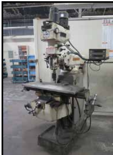
Lagun FTV-1 Vertical Mill w/ Mitutoyo DRO
