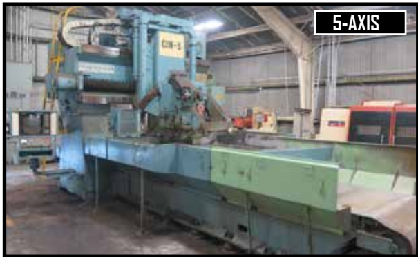
Cincinnati "30V-5Axis Bridge Profiler" 5-Axis CNC Vertical Machining Center w/ Acramatic 950 Controls, CAT-50 Spindle
