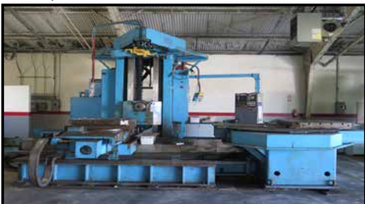
Ex-Cell-O "Work Center" XL-508/5 AXIS 2-Pallet 5-Axis CNC Horizontal Boring Mill w/ GE Fanuc 11M Controls, 30-Station ATC, CAT-50 Taper Spindle, 5 1/2" Spindle, 5 th Axis Thru Pallets, (2) 39 3/4" x 39 3/4" Pallets, Coolant.
