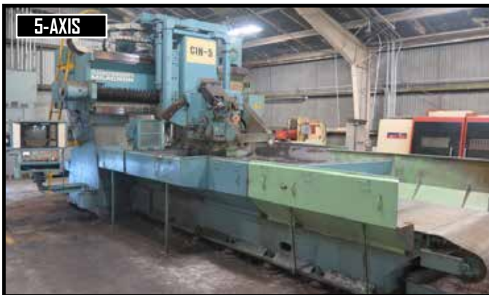
Cincinnati "30V-5Axis CNC Bed Mill w/ Acramatic 950 Controls, CAT-50 Spindle, 60" x 120" travels.
