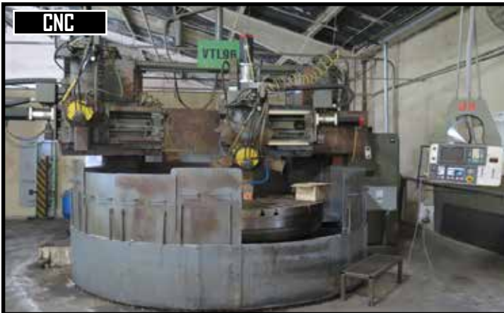
Betts 96" Twin Head CNC Vertical Turret Lathe w/ Fanuc 0-TT Controls
