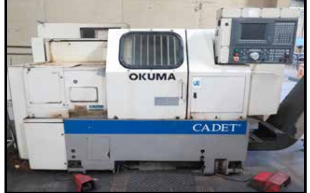
Okuma Cadet LNC-8C CNC Turning Center s/n 0806D703 w/ Okuma OSP700L Controls, 12-Station Turret, Hydraulic Tailstock, Jorgensen Chip Conveyor, Coolant.
