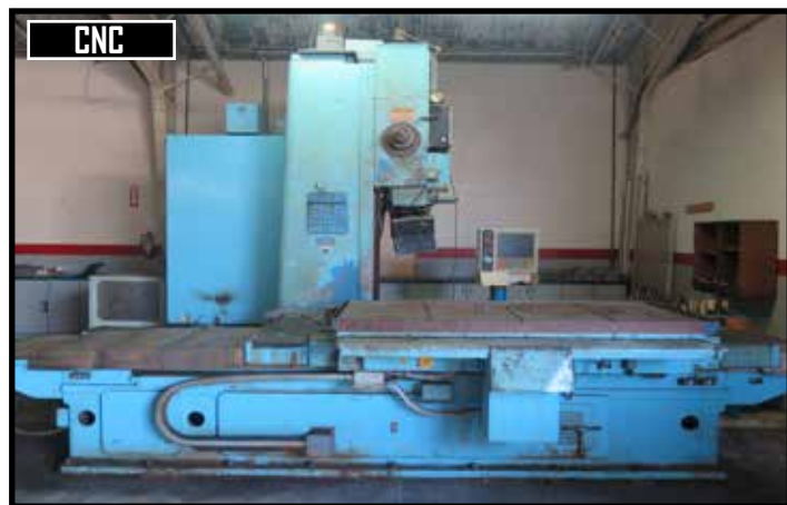
DeVlieg "Spiromatic Jigmill" 43H-72 CNC Jig Mill w/ MS-Tech CNC Controls
