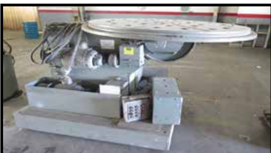
Aronson 21TS 5000 Lb Cap. Welding Positioner
