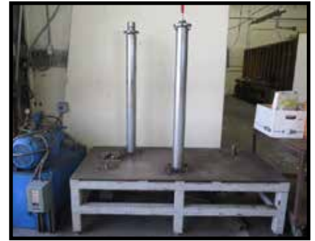
Custom Hydraulic J-Flange Expander
