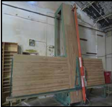
Rayco 76-10-V Vertical Panel Saw
