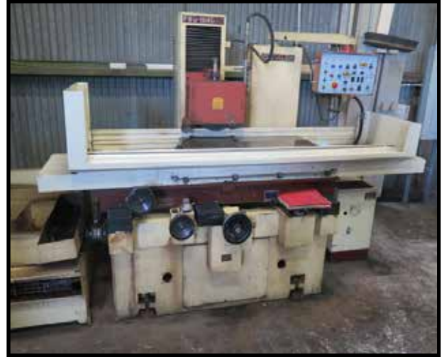
Chevalier FSG-1640AD 16" x 40" Automatic Surface Grinder s/n G478004 w/ Chevalier Controls, 16" x 40" Electromagnetic Chuck, Coolant and Filtration System.
