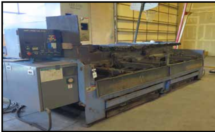
Takeda ABP-3100 "Auto Borer" Single Head CNC Plate / Beam Drill w/ Takeda CNC Controls
