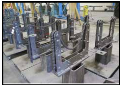
Chain Beam Rolls
