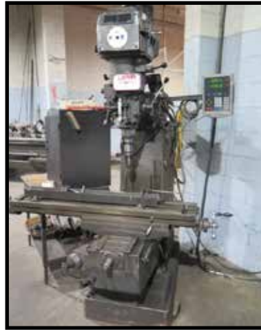
Lagun FTV-2 Vertical Mill w/ Newall C80 Programmable DRO
