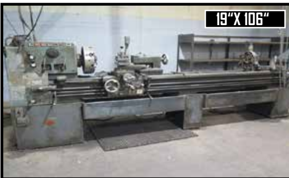
LeBlond 19" x 106" Lathe w/ 25-1000 Dial Change RPM, Inch Threading
