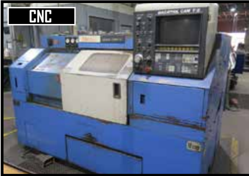
Mazak Quick Turn 15 CNC Turning Center w/ Mazatrol CAM T-2 Controls, Tool Presetter
