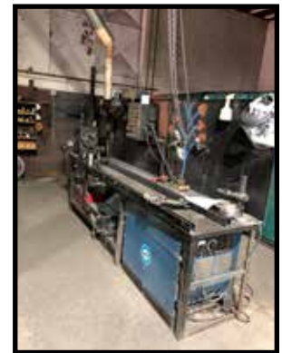
Custom Radial Welding System w/ Miller Deltaweld 450 CP-DC Welding Power Source
