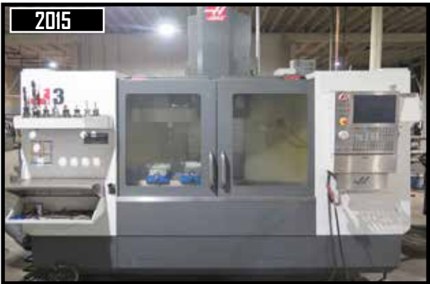
2015 Haas VF-3 CNC Vertical Machining Center w/ Haas Controls, 20-ATC, CAT-40, 8100 RPM, 30Hp Inline Spindle, Renishaw OTS Wireless Probe
