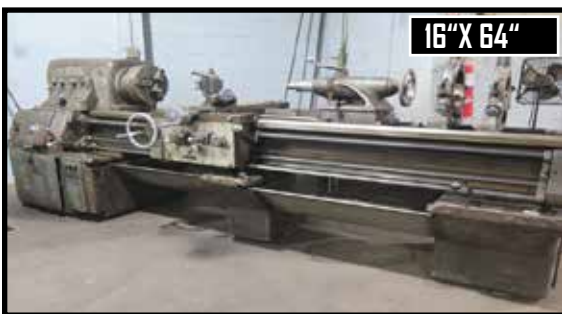
Monarch 16" x 64" Geared Head Lathe w/ Taper Attachment, 17-700 RPM
