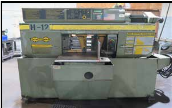
Hyd-Mech H-12 12" Automatic Hydraulic Horizontal Band Saw w/ Hyd-Mech Digital Controls
