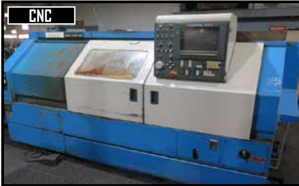
Mazak Quick Turn 28N CNC Turning Center w/ Mazatrol T32-2 Controls, Tool Presetter
