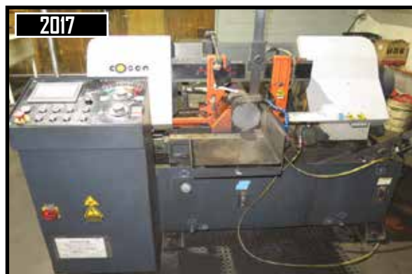
2017 Cosen C-260NC 11" Automatic Hydraulic Horizontal Band Saw w/ Cosen Digital Controls
