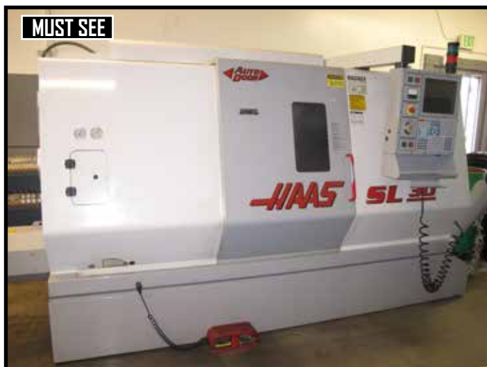
2000 HAAS SL-30T CNC LATHE, 12 STATION, TAIL STOCK, 10" CHUCK, CHIP AUGER, S/N 62990.
