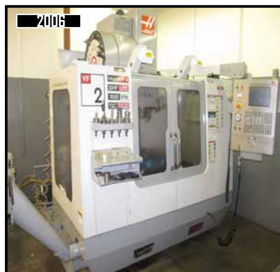
2006 HAAS VF-2B CNC VMC, 20HP, THROUGH SPINDLE COOLANT, SIDE MOUNT CHANGER, BT-40, 24 ATC, (XYZ) 30" X 16" X 20", S/N 1050360.
