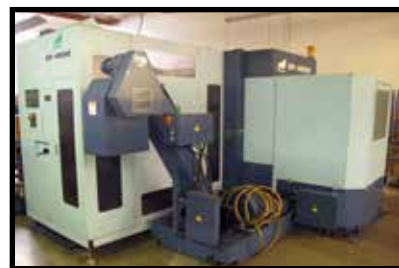
2000 MATSUURA ES-450H2-PC5 CNC HMC, AUTO 5 PALLET CHANGER, BT-40, 60 ATC, CHIPCONVEYOR, FANUC 18i-M CONTROL, PROBE, (XYZ) 17.71" X 15.74" X 15.74", S/N 000313947.
