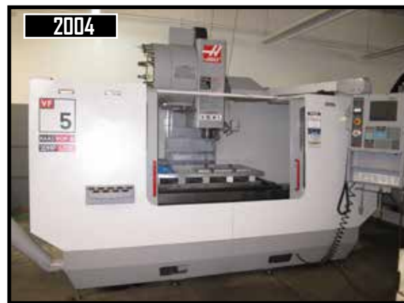
2004 HAAS VF5B/40 CNC VMC, 20 HP, SIDE MOUNT TOOL CHANGER, 24 ATC, BT-40, (XYZ) 50" X 26" X 25", S/N 38289.
