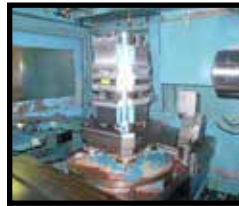
MATSUURA MAM-600H-PC2 CNC HMC, 2 PALLET CHANGER, BT-40, 60 ATC, CHIP CONVEYOR, (XYZ) 23.2" X 21.6" X 21.6", S/N 96071.
