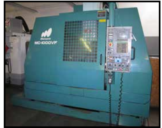
MATSUURA MC-1000VF CNC VMC, YASNAC i80 CONTROL, 40 TAPER, 30 ATC, (XYZ) 40" X 20" X 20", S/N 960211721.
