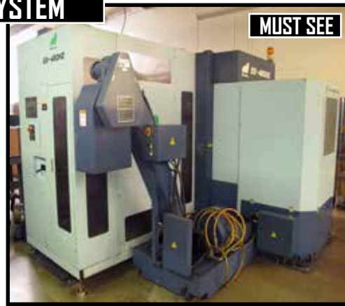
MATSUURA MAM-600H-PC2 CNC HMC, 2 PALLET CHANGER, BT-40, 60 ATC, CHIP CONVEYOR, (XYZ) 23.2" X 21.6" X 21.6", S/N 96071.
