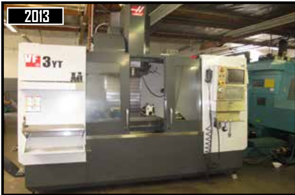
2013 HAAS VF3-YT CNC VMC, SIDE MOUNT TOOL CHANGER, BT-40, 24 ATC, PROBE, 4 TH AXIS READY, CHIP AUGER, (XYZ) 40" X 26" X 25", S/N 1107041.
