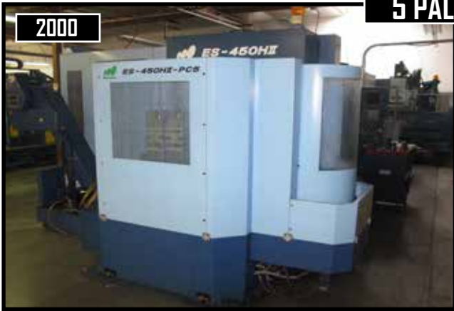
2000 MATSUURA ES-450H2-PC5 CNC HMC, AUTO 5 PALLET CHANGER, BT-40, 60 ATC, CHIP CONVEYOR, FANUC 18i-M CONTROL, PROBE, (XYZ) 17.71" X 15.74" X 15.74", S/N 000313947.
