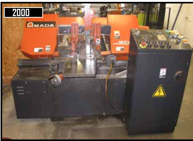
2000 AMADA HA-250W AUTO HORIZONTAL BAND SAW, AUTO FEED, 10" ROUND CUT CAP.
