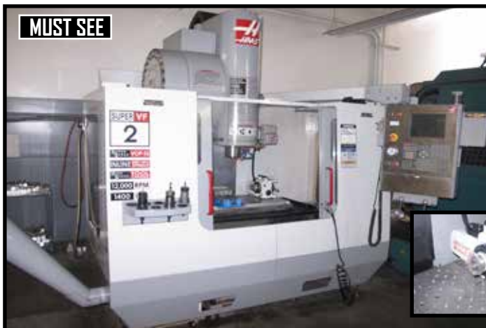
2004 HAAS VF2SS CNC VMC, 12,000 RPM, HI SPEED TOOL CHANGER, 4 TH AXIS READY, BT-40, 24 ATC, (XYZ) 30" X 16" X 20", S/N 38727.
