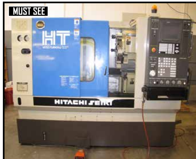
HITACHI SEIKI HT20J CNC TURNING CENTER, 12 STATION, SEICOS J CONTROL, TOOL SETTER, TAIL STOCK, 8" CHUCK, S/N 3851 HL.
