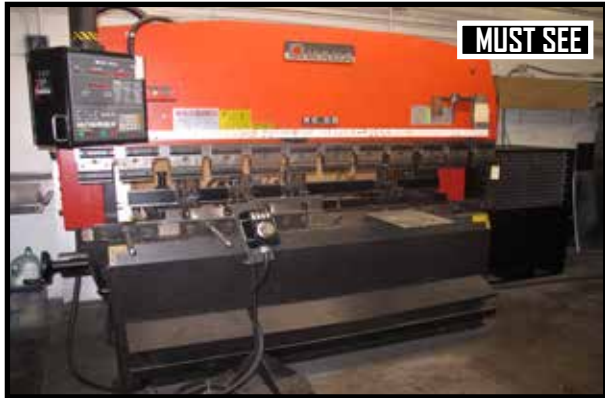
1990 AMADA RG-80, 98" X 80 TON CNC PRESS BRAKE W/ NC9EXII 3 AXIS CONTROL, S/N 50052.
