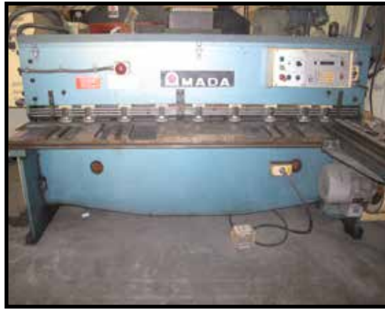
AMADA M-2045, MECHANICAL 73.74" X 3/16" POWER SHEAR, W/ CNC BACK GAGE, SQ ARM.
