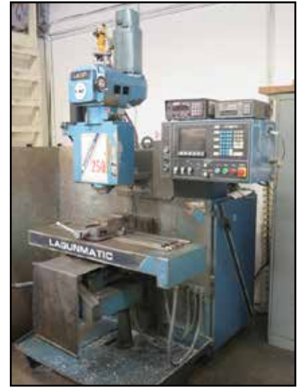
Lagun "Lagunmatic" 3-Axis CNC Vertical Mill w/ Delta 10CNC Controls, 40-Taper Spindle
