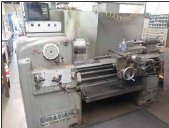
Graziano Tortona SAG-14 14" x 40" Gear-Gap Bed Lathe w/ Anilam Wizard 300Plus DRO
