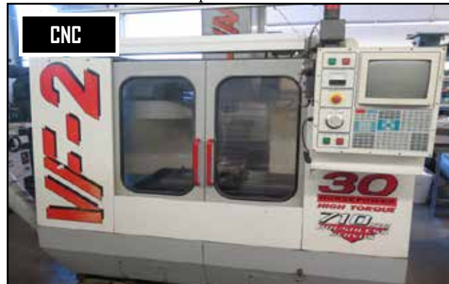
1998 Haas VF-2 4-Axis CNC Vertical Machining Center w/ 20-Station ATC, CAT-40 Spindle, 10,000 RPM, Thru Spindle Coolant, Rigid Tapping
