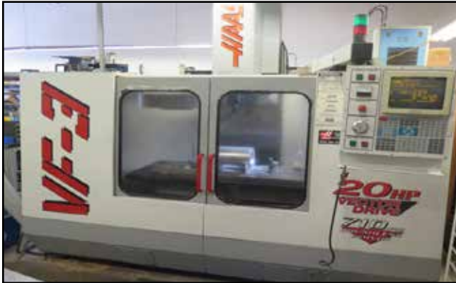
1997 Haas VF-3 4-Axis CNC Vertical Machining Center w/ 20-Station ATC, CAT-40 Spindle, 7500 RPM
