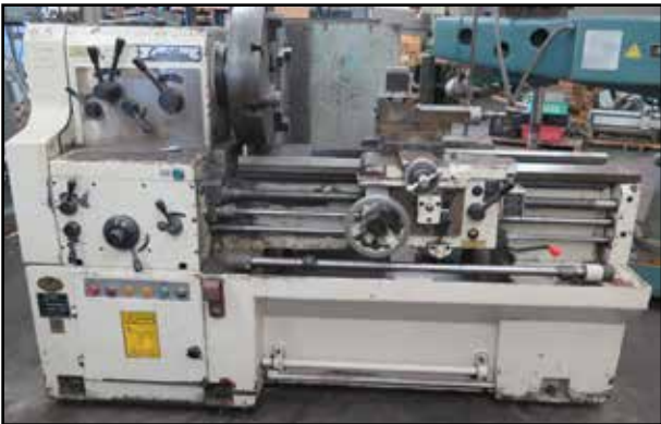
Cadillac 22" Geared Head Gap Bed Lathe w/ 25-1500 RPM
