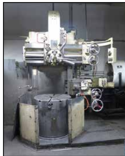
Bullard "Cut Master" 36" Vertical Turret Lathe w/ 6.6-240 RPM
