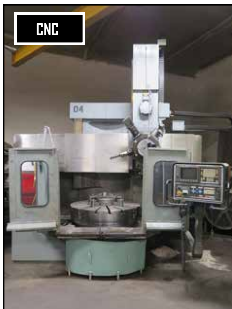
Giddings & Lewis 46" CNC Vertical Turret Lathe w/ Fanuc Series 0-T Controls
