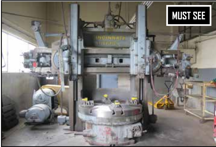
Cincinnati Hypro 52" Vertical Boring Mill w/ 57" Max Swing, 2.5-226 RPM
