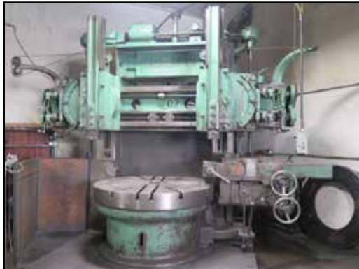
King 62" Vertical Boring Mill w/ 70" Max Swing, 1.7-83.4 RPM
