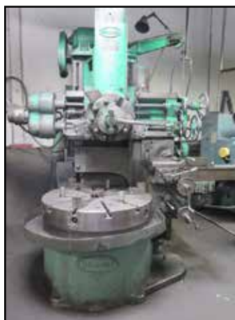
Bullard 42" Vertical Turret Lathe w/ 44" Max Swing, 168 Max RPM
