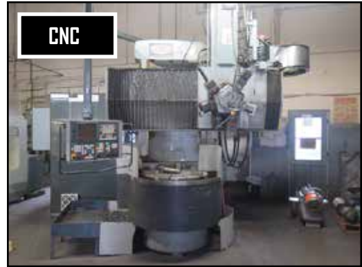
Bullard 36" CNC Vertical Turret Lathe w/ Fanuc Series 0-T Controls, 45" Max Swing
