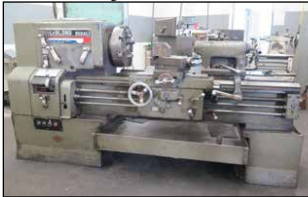
LeBlond Regal 22" x 40" Geared Head Lathe w/ 19-1500 RPM, Taper Attachment
