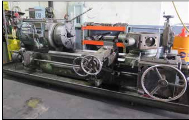
Warner & Swasey No. 4A Turret Lathe w/ 8-212 RPM, 8 1/4" Thru Spindle Bore
