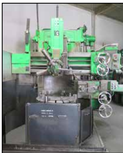
Bullard "Cut Master" 36" Vertical Turret Lathe w/ 40" Max Swing, 4.9-180 RPM
