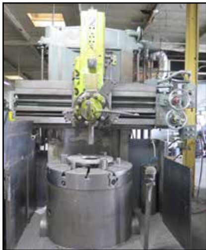
Bullard "Cut Master" 42" Vertical Turret Lathe w/ 56" Max Swing, 4.1-150 RP
