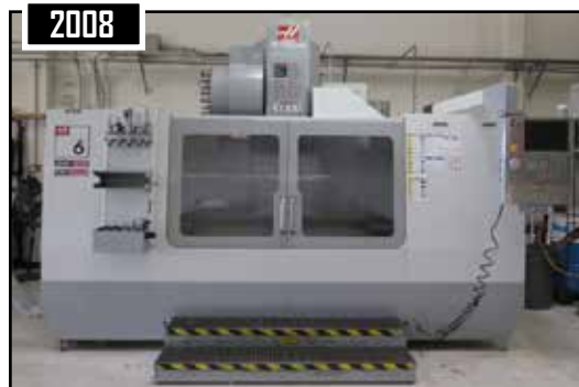
2008 2008 Haas VF-6/40 CNC Vertical Machining Center w/ 24-Station Side Mount ATC, CAT-40 Spindle,7500 RPM, Renishaw Wireless Probing System, Thru Spindle Coolant
