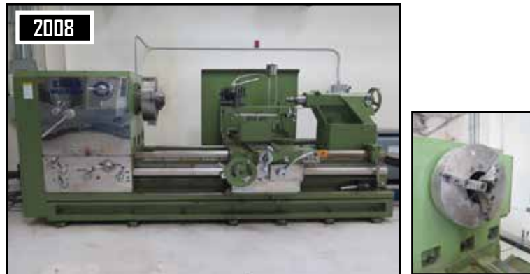
2008 2008 Eisen PS-4560 45” x 60” Geared Head Lathe w/ 6” Thru Spindle Bore, 7-700 RPM, Inch/mm Threading
