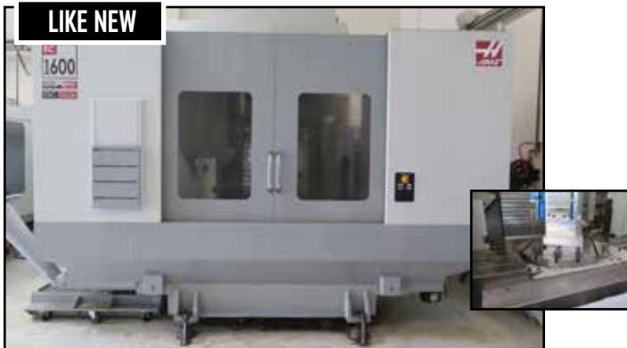
LIKE NEW 2009 Haas EC-1600-4X 4-Axis CNC Horizontal Machining Center w/ 30-Station Side Mount ATC, CAT-50 Taper Spindle, 6000 RPM, Full 4 th Axis Through 29 ½” Built-In 4 th Axis Rotary, Renishaw Wireless Probing System, Rigid Tapping, Thru Spindle Coolant
