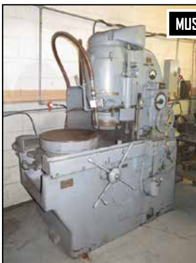
Blanchard No. 11 20" Blanchard Grinder w/ Blanchard Controls, 20" Magnetic Chuck, 11" Grinding Head
