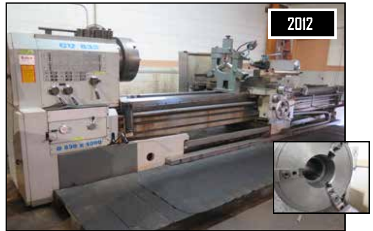
2012 Lion CU-832 33" x 157" Geared Head Gap Bed Lathe w/ 6" Thru Bore, 5.6-1000 RPM, Taper Attachment, 20" 3-Jaw Chuck
