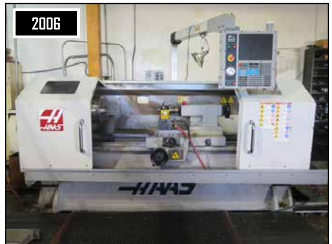
2006 Haas TL-3 Tool Room Lathe w/ Haas Controls, 1800 RPM, Tailstock, 12 1/2" 3-Jaw Chuck
