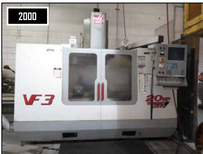
2000 Haas VF-3 4-Axis CNC Vertical Machining Center w/ Haas Controls, 20-Station ATC, BT-40 Taper Spindle, 10,000 RPM
