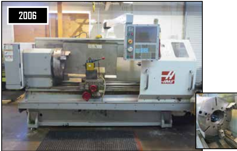
2006 Haas TL-3B Big Bore Tool Room Lathe w/ Haas Controls, 8 1/2" Thru Spindle Bore, 650 RPM, Rigid Tapping, 25" 3-Jaw Front and Rear Chuc
