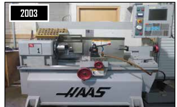
2003 Haas TL-1 Tool Room Lathe w/ Haas Controls, 1800 RPM, Tailstock, 8" 3-Jaw Chuck
