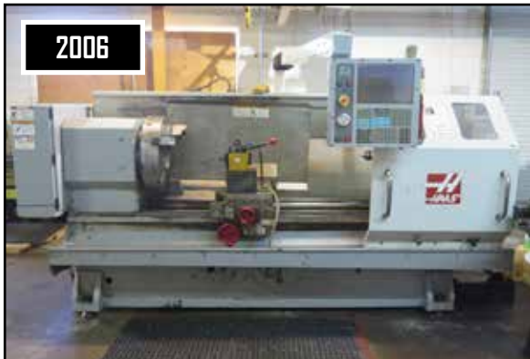
2006 Haas TL-3B Big Bore Tool Room Lathe w/ Haas Controls, 8 1/2" Thru Spindle Bore, 650 RPM, Rigid Tapping, 25" 3-Jaw Front and Rear Chucks
