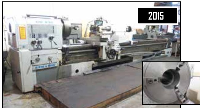
2015 Lion CU-832 33" x 157" Geared Head Gap Bed Lathe w/ Newall PD700 DRO, 6" Thru Spindle Bore, 5.6-1000 RPM, Taper Attachment
