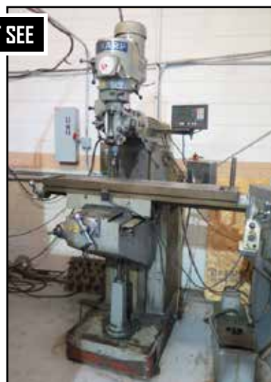
Sharp Vertical Mill w/ Newall Topaz DRO, 60-4500 RPM, Universal Kwik-Switch Spindle
