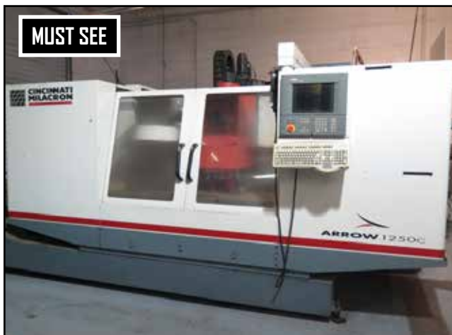
1998 Cincinnati Milacron Arrow 1250C CNC Vertical Machining Center w/ Acramatic 2100 Controls, Hand Controller, 21-Station ATC, 40-Taper Spindle
