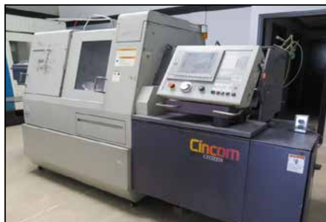
2001 Citizen Cincom M-12 CNC Twin Spindle Screw Machine
