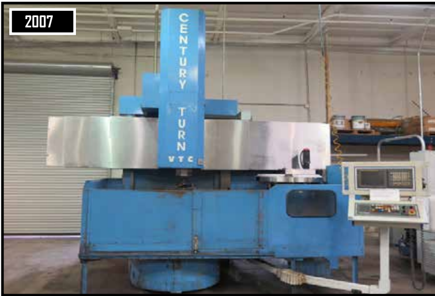
2007 New Century "Century Turn VTC" 56" CNC Vertical Turning Center w/ Fanuc 18i-T Controls, 12-Station ATC, Sandvik C-8 Tooling
