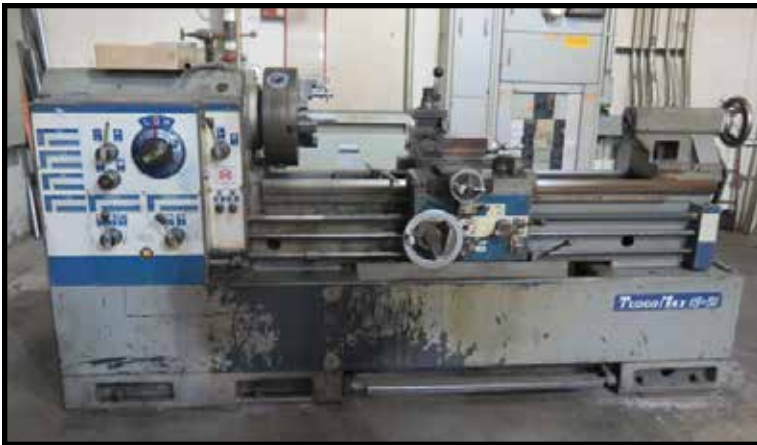
TudorMax 19" x 51" Gear-Gap Lathe w/ 35-1800 RPM
