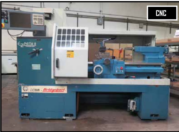
Romi Bridgeport EZ-Path II MS-20 CNC Lathe w/ EZ-Path CNC Controls, 20 1/2" x 40" Cap., 4-3500 RPM
