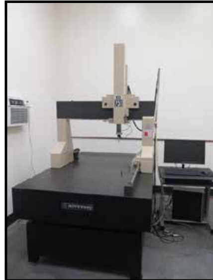
Mitutoyo B251 CMM Machine w/ Renishaw PH1 Probe Head
