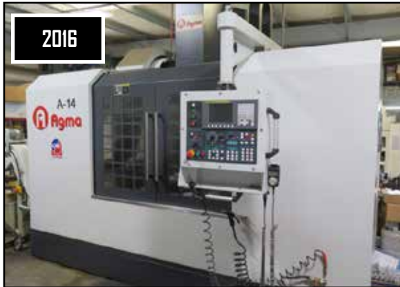
2016 Agma A-14 4-Axis CNC Vertical Machining Center w/ Fanuc 0i-MF Controls, 24-Station Side Mount ATC, CAT-40 Taper Spindle, 12,000 RPM Direct Drive Spindle, Rigid Tapping
