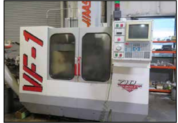
1997 Haas VF-1 CNC Vertical Machining Center s/n 9848 w/ Haas Controls, 20-Station ATC, CAT-40 Taper Spindle, 7500 RPM
