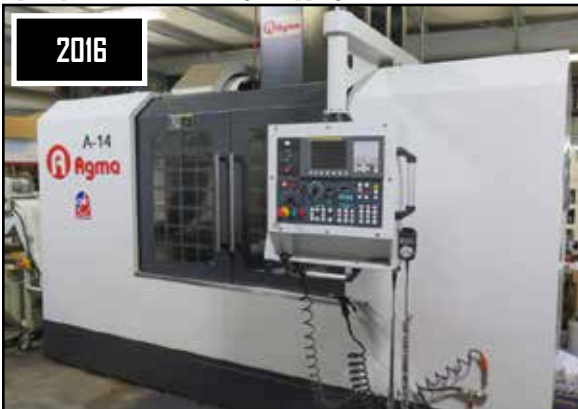
2016 Agma A-14 4-Axis CNC Vertical Machining Center w/ Fanuc 0i-MF Controls, 24-Station Side Mount ATC, CAT-40 Taper Spindle, 12,000 RPM Direct Drive Spindle, Rigid Tapping
