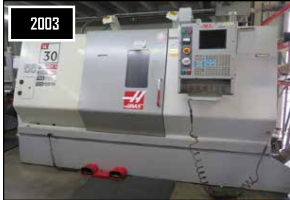
2003 Haas SL-30 CNC Turning Center w/ Haas Controls, Tool Presetter, 12-Station Turret, 3400 RPM, 3" Thru Spindle Bore, 30Hp, Tailstock
