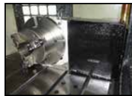
2016 Agma A-14 4-Axis CNC Vertical Machining Center w/ Fanuc 0i-MF Controls, 24-Station Side Mount ATC, CAT-40 Taper Spindle, 12,000 RPM Direct Drive Spindle, Rigid Tapping
