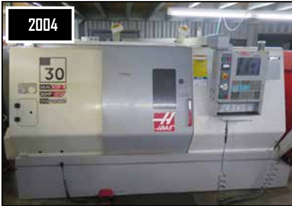
2004 Haas SL-30 CNC Turning Center w/ Haas Controls, Tool Presetter, 12-Station Turret, 3400 RPM, 3" Thru Spindle Bore, 30Hp, Rigid Tapping
