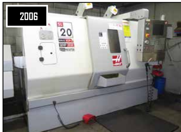
2006 Haas SL-20 CNC Turning Center w/ Haas Controls, Tool Presetter, 10-Station Turret, 4000 RPM Baldor Spindle Motor, 20Hp, Rigid Tapping, 10mm Pitch Ball Screws
