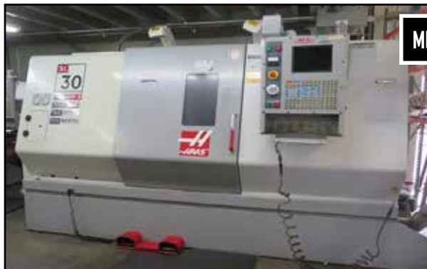
2003 Haas SL-30 CNC Turning Center w/ Haas Controls, Tool Presetter, 12-Station Turret, 3400 RPM, 3" Thru Spindle Bore, 30Hp, Tailstock
