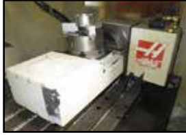
1997 Haas VF-4 5-Axis Capable CNC Vertical Machining Center w/ Haas Controls, 20-Station ATC, CAT-40 Taper Spindle, 7500 RPM, 4 th and 5 th Axes Drive Controllers
