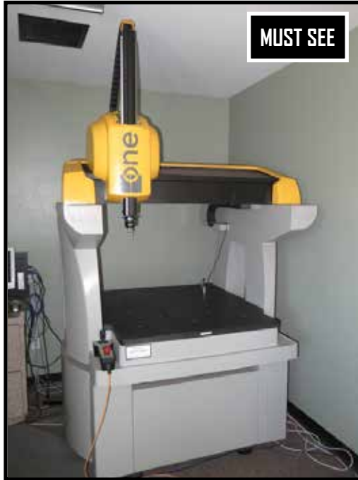
2003 Brown & Sharpe "ONE 775" CMM Machine w/ Hand Held Drive Controller, Renishaw MH20i Motorized Probe Head, PC-DMIS CAD+ Software with Scanning Option
