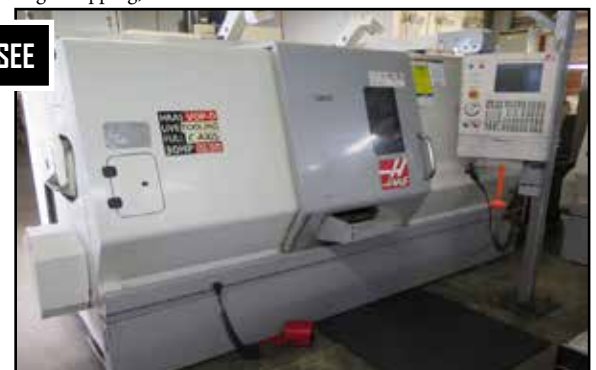
2006 Haas SL-30 CNC Live Turret Turning Center w/ Haas Controls, Tool Presetter, 12-Station Live Turret, (2) Radial and Axial Live Tooling, 3400 RPM
