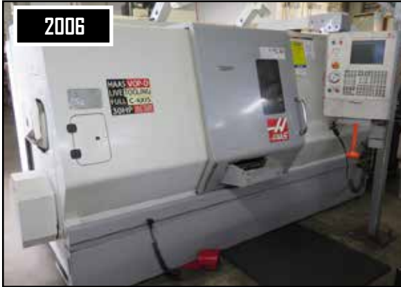
2006 Haas SL-30 CNC Live Turret Turning Center w/ Haas Controls, Tool Presetter, 12-Station Live Turret, (2) Radial and Axial Live Tooling, 3400 RPM
