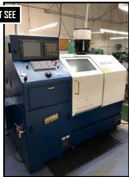
2003 HARDINGE QUEST GT27SP CNC GANG TOOL LATHE, W/ FANUC 21i-TB CONTROL, COOL JET SYSTEM, S/N MG-102.
