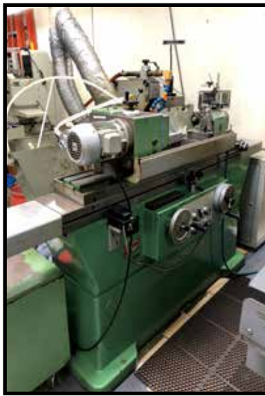
TCHUDIN HTG 610 CYLINDRICAL GRINDER W/ DRO, S/N 76-120
