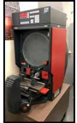
STARRETT HB400 OPTICAL COMPARATOR W/ QUADRA CHEK 2000 CONTROL, S/N 3427.
