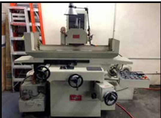
KENT MODEL KGS-300AHD, AUTOMATIC HYD. SURFACE GRINDER, S/N 840205-3.
