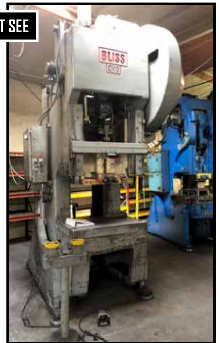
Bliss C-110, 110 Ton Obi Punch Press, 6" Stroke, Air Clutch, 21" Shut Height, Palm Button Controls. (Note: This Machine Is Sold As Is With No Current Updated Controls)
