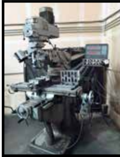
SuperMax Vertical Mill 42" x 9" table Chrome Ways, Accu-Rite II DRO, Power Feed.
