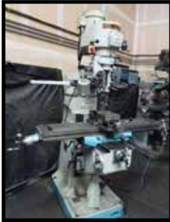
1996 YC1 SuperMax Vertical Mill 49 x 9 Table, Chrome Ways, Accu-Rite DRO, Power Feed.
