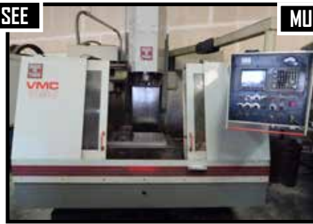
Tree Vmc 1050E Vertical Machining Center, 24 Position Tool Changer 50 x 24Table S/N912932008 24x40 Travel, Axis X 40Y 20 Z 25&8,000 RPM Spindle, Dynapath Delta Control.
