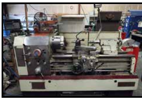
Acer Dynamic 1740G Engine Lathe 17" Series Gap Lathe, 1 1/2 Thru Hole 9" Chuck, NewAll DRO.
