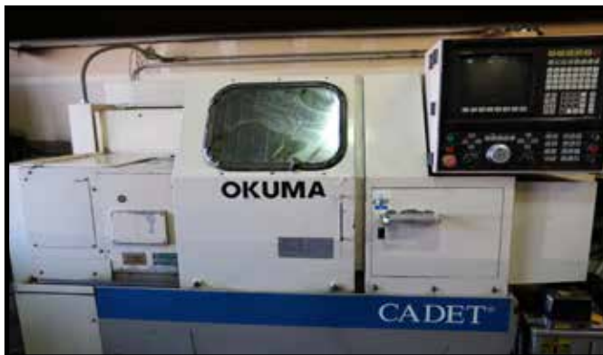
Okuma Cadet LNC-8C CNC Turning center, 12-Station turret, Tail-stock, Spindle Nose, 9" Chuck, S/N 0711D263 Okuma Control, Chip Conveyor.
