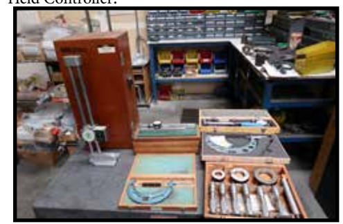
Partial View of Inspection Tools, Pin Gages, Calipers, Height Master, Granite Plates.
