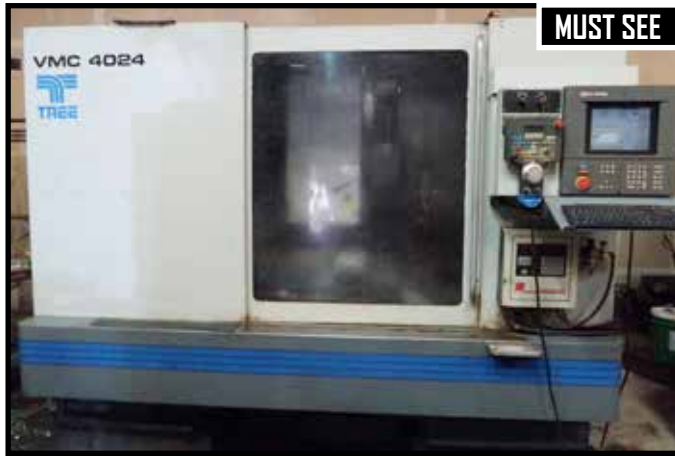
Tree VMC 4024 Vertical Machining Center, 20 Position Tool Changer, 51" x 24" Table, S/N 990981359 Axis X 40" Y 24" Z 25" 10,000 RPM Spindle, Coolant Thru, TPC-2100 Control Hand Held Controller.
