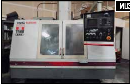
Tree Vmc 1050E ZPS Vertical Machining Center, 24 Position Tool Changer 50x 24x40 Travel, Axis X 40 Y 20 Z 25 8,000 RPM Spindle, Dynapath Delta Control
