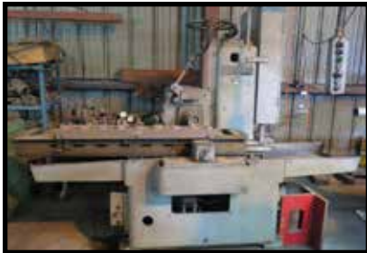
Sundstrand mdl. 22 "Rigidmill" Horizontal Boring Mill
