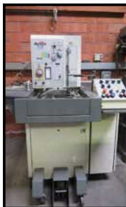
Sunnen Eclipse EC-3500-D Honing Machine w/ Power Stroke, Auto Sizing, Pneumatic Holding
