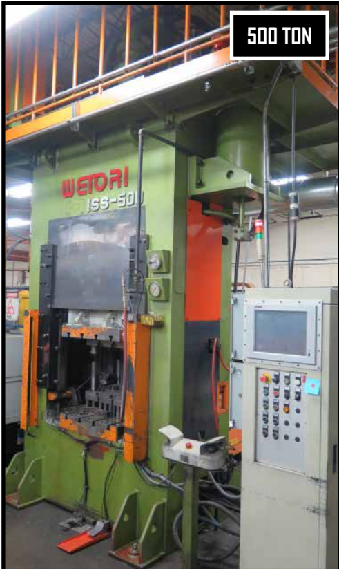
Wetor 165-50 500 Ton Hot Forging Hydraulic Press w/ Phoenix Contact Touch Screen Controls, 40 Ton Pull-Out Force
