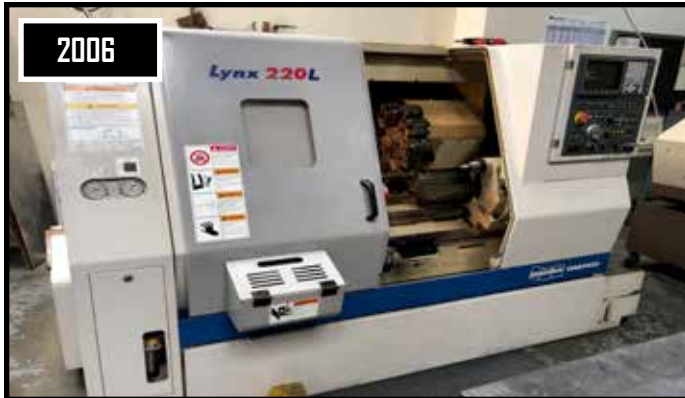
2006 Doosan Daewoo Lynx 220LC CNC Turning Center, 8" Chuck, Tail Stock, Fanuc Control, s/n 12200994.
