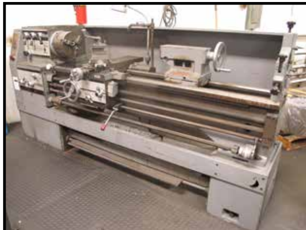
JET 18 X 60 ENGINE LATHE WITH 10" 3 JAW CHUCK, 40 TO 160 RPM
