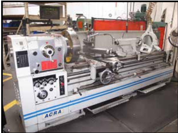
ACRA 22" X 90" GAP ENGINE LATHE, W/ 4" THRU HOLE, INCH / METRIC THREADING
