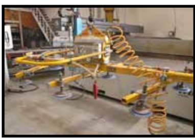
ANVER VIF-57 900 LB CAPACITY VACUUM LIFT.
