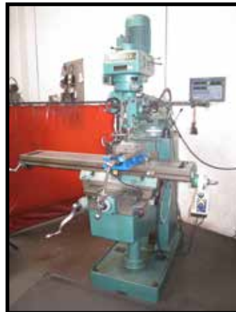
GRIZZLY VERTICAL MILLING MACHINE, MOD G9904, NEWALL DRO, POWER FEED TABLE, 10 X 54 TABLE.
