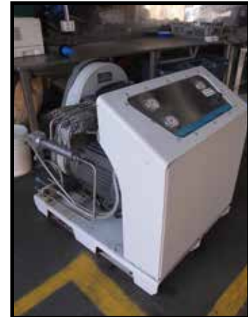
FLOW 52,000 PSI HYPLEX PRIME PUMPS, MODEL 050051-1-1-1-1-1, S/N 715-15493.
