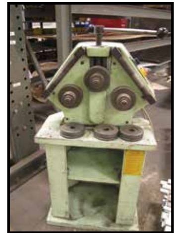
BCR MODEL RBM 2-30, MECHANICAL 3 ANGLE ROLLS, S/N 9G3002.
