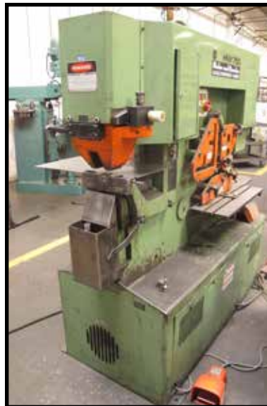
MUBEA MODEL HTW-750, HYD 75 TON IRON WORKER.
