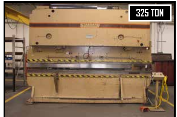
STANDARD MODEL AB325-12, 12FT X 325 TON HYD PRESS BRAKE, PALM BUTTON CONTROLS, HYDRAULIC, S/N 297583.
