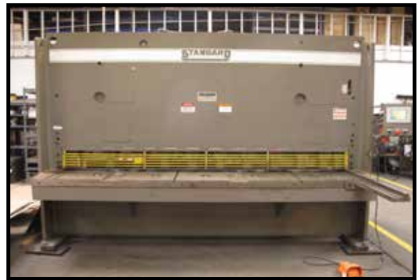
STANDARD MODEL AS500-10, 10FT X 0.5" CAPACITY HYD POWER SHEAR W/ SQUARING ARM, SIEMENS CNC TOUCH PANEL BACK GAGE, S/N F10091772.
