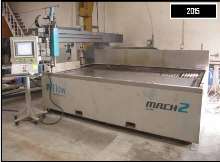
2015 FLOW MACH 2 CNC WATER JET MODEL M2- 2031B, W/ 2017 JET EDGE IP6030 60,000 PSI INTENSIFIER PUMP, 6FT X 10FT TABLE, COLOR MONITOR SCREEN S/N 150199
