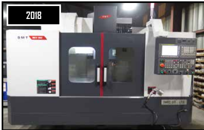
2018 SMT Samsung Machine Tools MCV500 CNC Vertical Machining Center w/ Fanuc Oi-MFControls, 30-ATC, CAT-40
