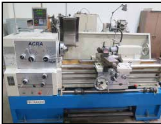
Acra FEL-1640 GNX 16" x 40" Geared Head Gap Bed Lathe w/ Newall C80 DRO
