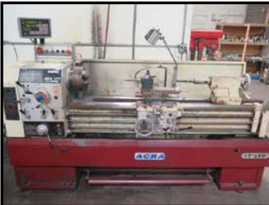
Acra 17" x 60" Geared Head Gap Bed Lathe w/ SWC SDS6-2V DR0
