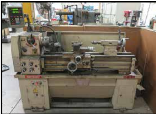
Ganesh GT-1440 14" x 40" Geared Head Gap Bed Lathe w/ Newall C80 DR0
