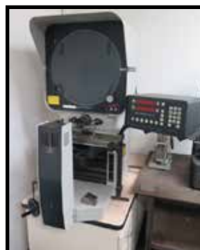
Deltronic DH216-612R 15" Optical Comparator w/ Deltronic 612-R DRD
