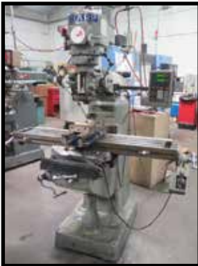
2007 Sharp LMV-50 Vertical Mill w/ Newall C80 DRD, 3Hp Motor
