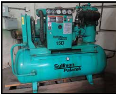
Sullivan Palatek 15DTW 15Hp Rotary Air Compressor
