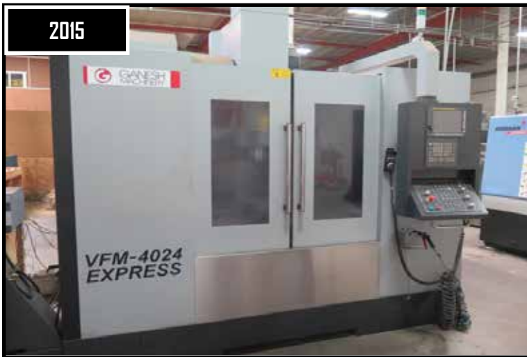
2015 Ganesh VFM-4020 "Express" CNC Vertical Machining Center w/ Fanuc Oi-MF Controls, 30-ATC, CAT-40
