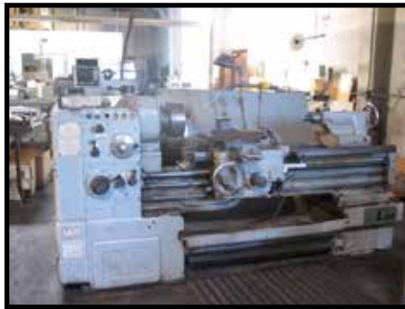
WASINO MODEL 6000 ENGINE LATHE, WITH NEWALL DR0, 3 JAW CHUCK.
