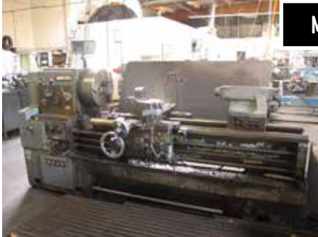
MORI SEIKI MH1500G, 24" X 60" GAP ENGINE LATHE WITH 16" 3 JAW CHUCK, 3" THRU SPINDLE HOLE,
