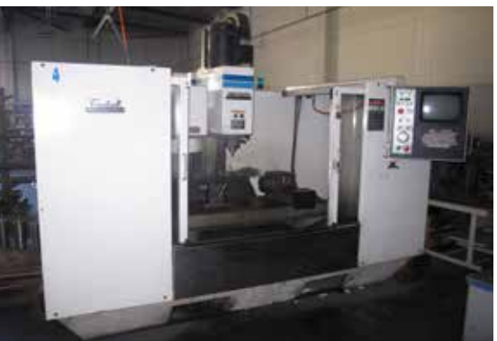
1993 FADAL VMC 4020HT CNC VMC, CT-40, 20 ATC, 4 TH AXIS ROTARY, S/N 9304224.
