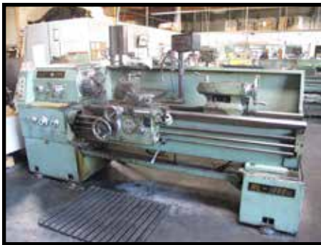
MIGHTY TURN ML-1860GL, 18" X 60" GAP ENGINE LATHE WITH DR0, 3 JAW CHUCK.
