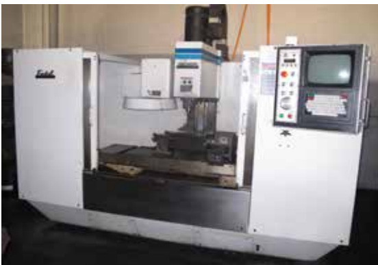
1995 FADAL VMC 4020HT CNC VMC, CT-40, 20 ATC, W/ VH65 4 TH AXIS ROTARY, S/N 9510941
