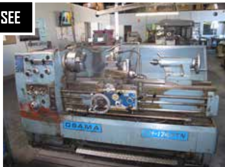
OSAMA CH-1740TN, 17" X 40" GAP ENGINE LATHE WITH SONY DRO, 3 JAW CHUCK.
