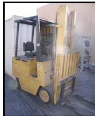
TOWMOTOR 4000 LB ELECTRIC FORKLIFT WITH CHARGER
