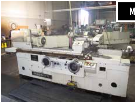
1997 MIGHTY M1340 UNIVERSAL OD GRINDER, 13" X 40" CAPACITY, WITH DRO, S/N 97010.
