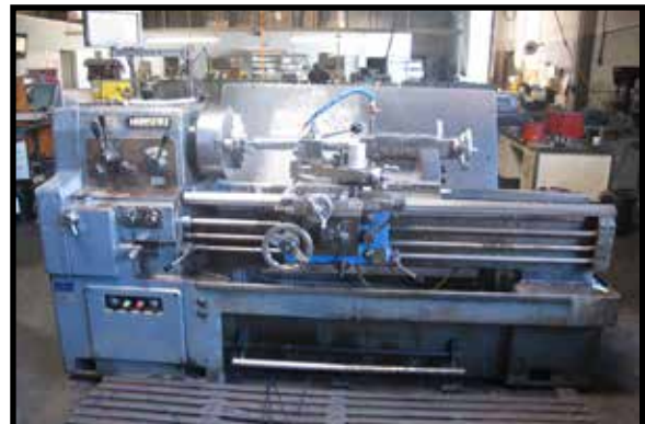
MORI SEIKI MS1250G, 17" X 50" GAP ENGINE LATHE, WITH NEWALL DRO.
