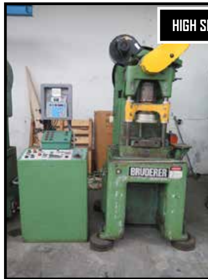
Bruderer BTSA-30 30-Ton High Speed Stamping Press w/ Bruderer ElectroCam Plus 5000 Controls
