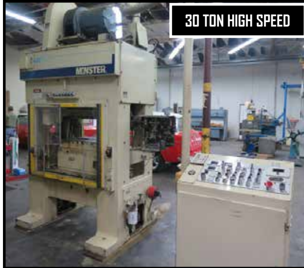
Minster Pulsar 30 type TR2-30 30-Ton High Speed Stamping Press w/ Minster Controls
