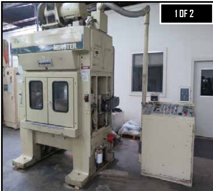
Minster Pulsar 30 type TR2-30 30-Ton High Speed Stamping Press w/ Minster and Die Check Controls
