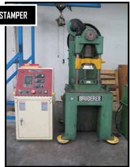
Bruderer BTSA-30 30-Ton High Speed Stamping Press w/ Wintriss Clutch and Brake Controls
