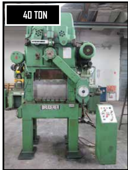
Bruderer BTSA40 40-Ton High Speed Stamping Press w/ Die Protection Controls
