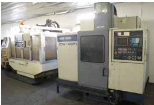
Kitamura Mycenter 3X CNC VMC, Yasnac Control, 10,000 RPM, 40 Taper, 20 ATC and Mori Seiki MV-40M CNC VMC, with Fanuc Control, 40 Taper.
