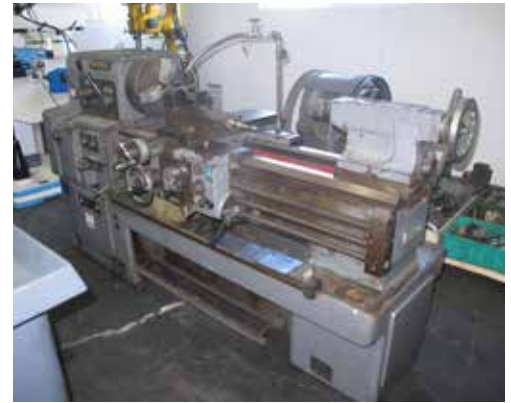
Webb 17" Gx40" 17" x 40" Geared Head Gap Bed Lathe s/n LS7909-06 w/ 38-1800 RPM, Inch Threading, Tailstock, KDK Tool Post, 12" 3-Jaw Chuck, Coolant
