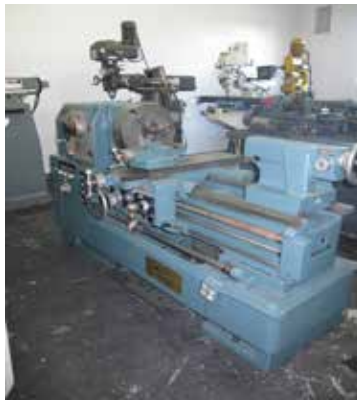
Chinhung CH94008 22" x 39" Geared Head Gap Bed Lathe w/ 13-1200 RPM, 4" Thru S spindle Bore, Tailstock, 16" 3-Jaw Chuck.
