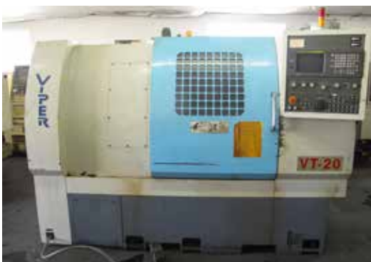
2002 Viper VT-20 CNC Lathe with Fanuc 18-T control, 12 Position Turret, 8" Chuck, Chip Conveyor. 8408 2005 Storm VM
