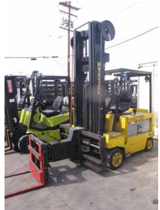
Hyster N30AH 1700 Lb Cap Narrow Isle Swing Mast Forklift s/nB210V01533P w/ Momotrol Gears, 256" Lift Height, Cushion Tires.
