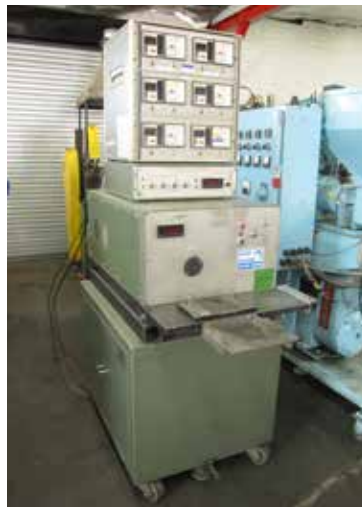
C.W. Brabbender type EPLV5502 Electronic Plasti-Corder Torque Rheometer Lab Mill 8" Rubber Mill. w/6 Zones
