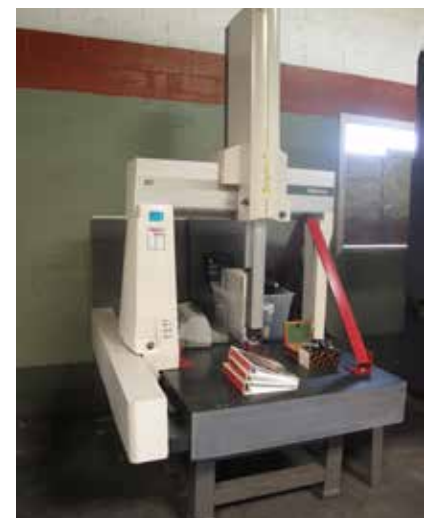
Mitutoyo Bright-M-9 mdl. M-710 CMM Machine s/n BC000112 w/ Renishaw PH8 Probe Head, GEOMeasure Software, 43 1/2" x 64" x 8 1/2" Granite Table.
