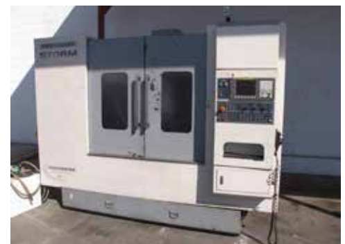
2005 Storm VMV-1020 CNC VMC with Fanuc Oi-MC Control, 24 ATC, 40 Taper, Chip Conveyor.
