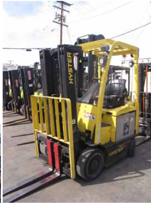
Hyster E50XN-27 4850 Lb Cap Electric Forklift s/n 268N03571H w/ 3-Stage Mast, 189" Lift Height, Side Shift, Cushion Tires, 3223 Hours.
