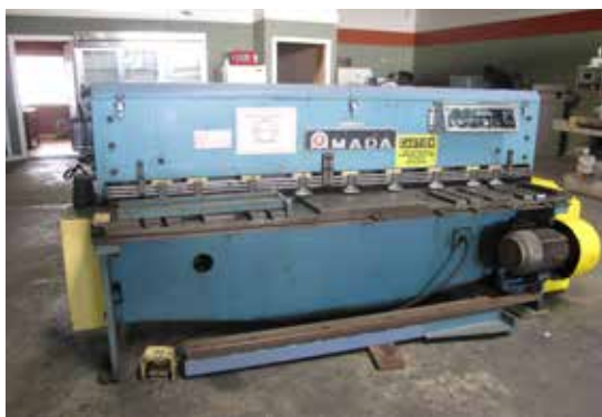
Amada M2045 3/16" x 78" Power Shear s/n 2401093 w/ 80" Squaring Arm, Front Supports, 60 Strokes/Min.
