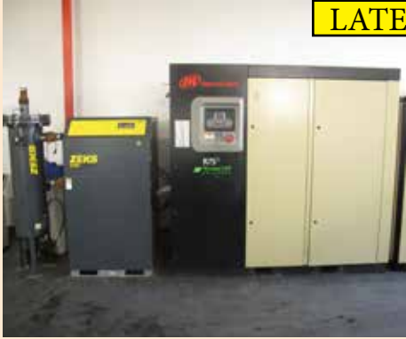
Ingersoll Rand R75n "Nirvana VSD Efficient" mdl. R75N-A145 100Hp Rotary Air Compressor s/n NK1240U12150 w/ DigitalControls.
