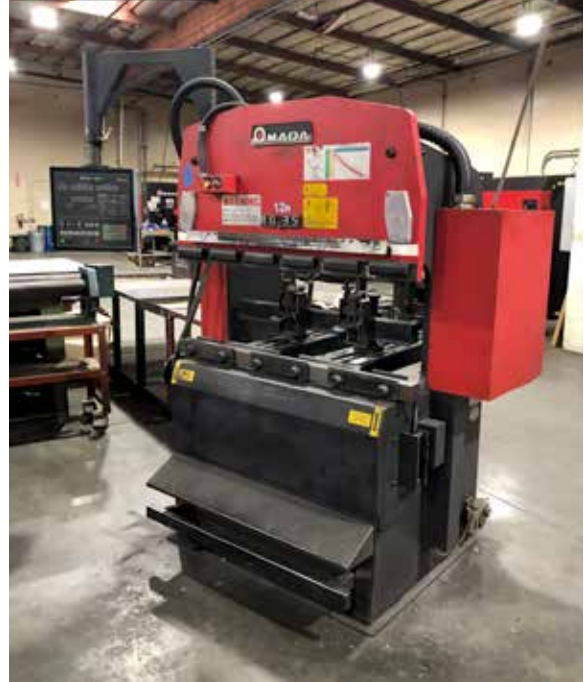
Amada RG-35S 35 Ton x 48" CNC Press Brake, w/ NC9EX Control
