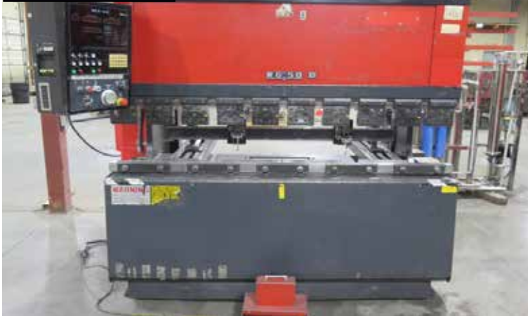
Amada RG-50D 50 Ton x 78" CNC Press Brake, w/ NC9EX Control
