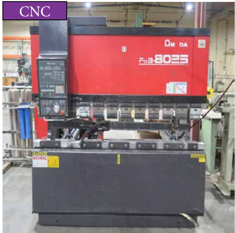
Amada FBD-8025 80 Ton x 98" CNC Press Brake w/ NC9EX Control
