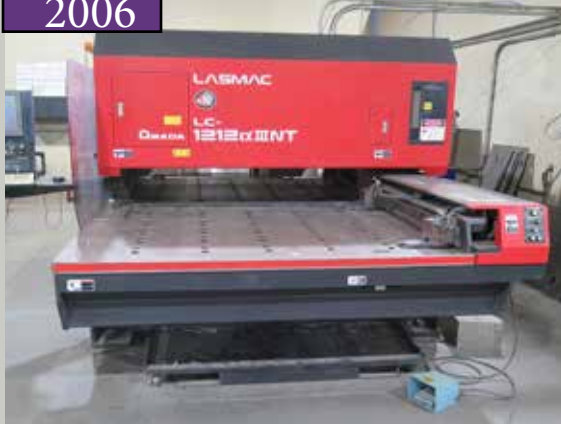
2006 Amada Lasmac LC-1212 cxIIIINT 2kW Laser Contour Machine
