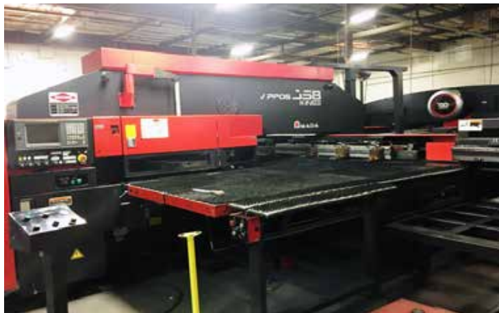
1998 Amada Vipros 358 King II CNC Turret Punch Press, 30 Ton, 58 Tool, 2 AI, Fanuc 18 - P Control
