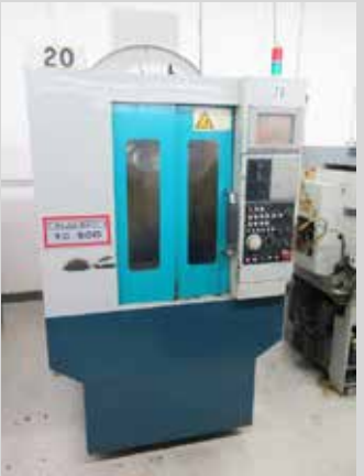
2000 Akira Seiki TC500 CNC Drilling/Tapping Machine w/ Mitsubishi Controls
