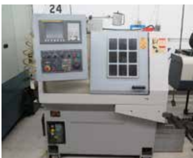
Ganesh CS-32T CNC Gang Tool/ Turret Turning Center w/ Fanuc series i-Mate-TC Controls
