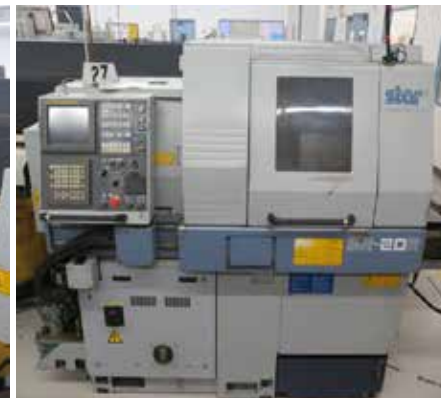
Star SR-20R Twin Spindle CNC Screw Machine w/ Fanuc Series 18i-T Controls
