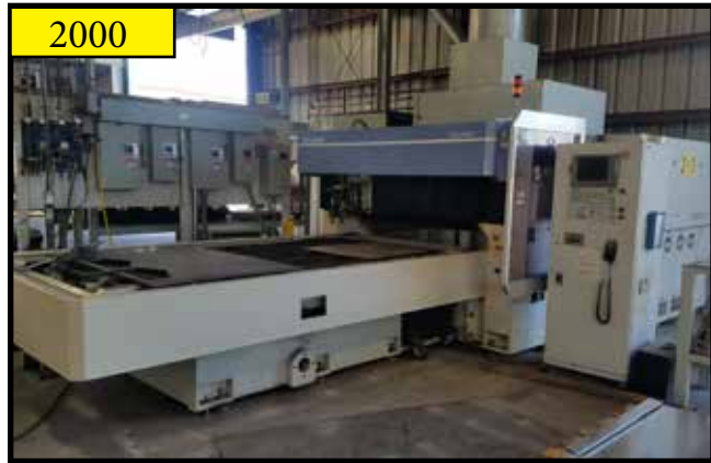
2000 MITSUBISHI CNC LASER PROCESSING MACHINE MOD. 2512HD II ,CO2 3 AXIS (2600MM , 1250MM, 150 X-Y-Z) WITH MITSUBISHI LC20B CONTROL, 4' X 8' TABLE, S/N1025HDII037, LASER UNIT ML3036D 3.6KW THERMAL CARE ACCUCHILLER,
