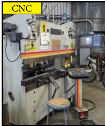
1995 ACCUPRESS MOD. 7606 60 TON, 6 FEET CNC PRESS BRAKE S/N 2913W/ACCUPRESS CONTROL, BACK GAGE
