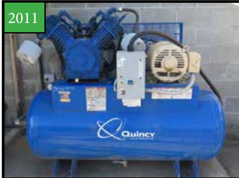
2011 QUINCY QT-15 15HP HORIZONTAL AIR COMPRESSOR
