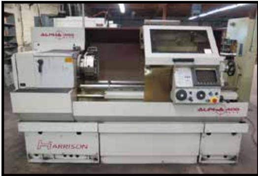
1998 HARRISON "ALPHA 400 PLUS" 16" X 52" CNC LATHE W/ HARRISON-GE FANUC CONTROLS
