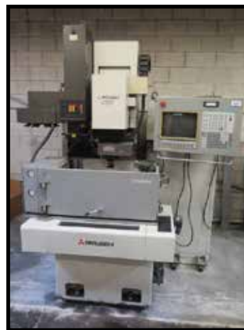
MITSUBISHI V25F CNC DIE-SINKER EDM MACHINE W/ C11G35 CONTROLS
