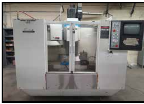
FADAL VMC40 4-AXIS CNC VERTICAL MACHINING CENTER W/ CNC88HS CONTROLS, 21-ATC, CAT-40
