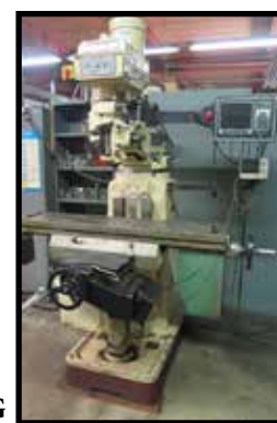
FADAL VMC40 4-AXIS CNC VERTICAL MACHINING CENTER W/ CNC88HS CONTROLS, 21-ATC, CAT-40
