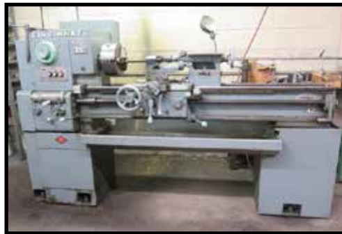
CINCINNATI 15" X 48" GEARED HEAD LATHE W/ 53-1800 DIAL HYDRASHIFT RPM
