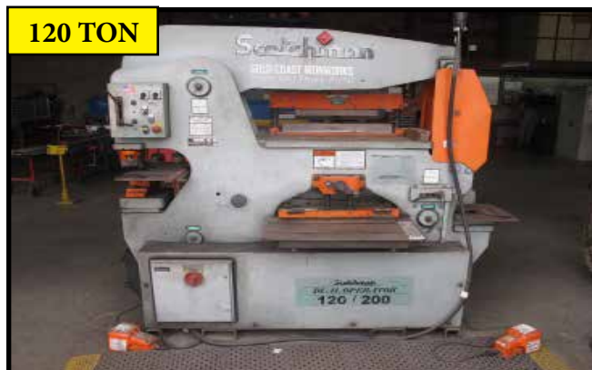
SCOTCHMAN 120 TON DUAL OPERATOR HYDRAULIC IRON WORKER, MODEL DO-120/200-24M WITH PUNCHES AND DIES
