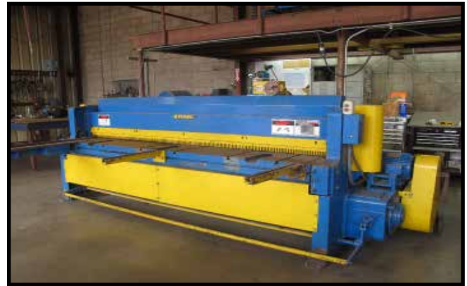
WYSONG MODEL 1010, 10FT X 10 GA MECHANICAL POWER SHEAR WITH FRONT OPERATED BACK GAGE, S/N P32-1036.
