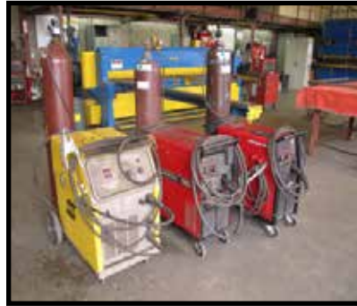
PARTIAL VIEW OF ESAB AND LINCOLN MIG WELDERS.
