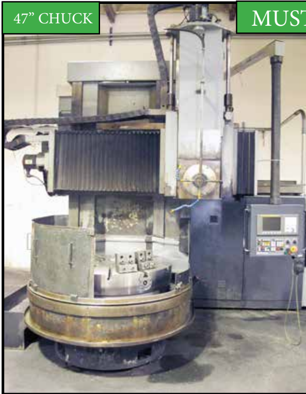
SUMMIT 47" CHUCK CNC VTL WITH FANUC OI-TD CONTROL, 4 JAW CHUCK, 4 POSITION TURRET, 50" SWING.
