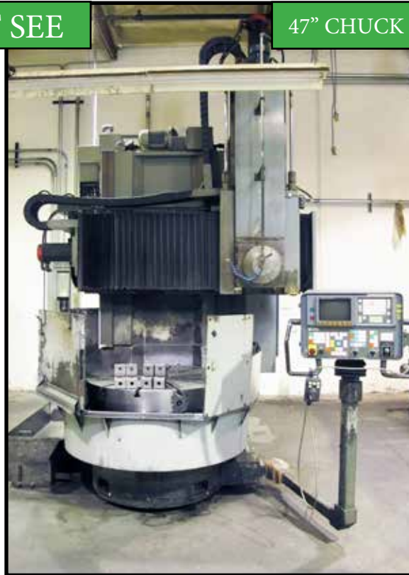
SUMMIT 47" CHUCK CNC VTL WITH FANUC OI-TD CONTROL, 4 JAW CHUCK, 4 POSITION TURRET, 50" SWING.
