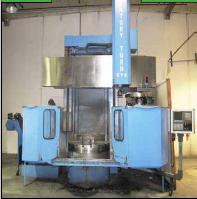
2012 (REMAN) NEW CENTURY 56" CHUCK CNC VTL W/ 12 STATION ATC, 70" SWING, FANUC Oi-TD CONTROL, 4 JAW CHUCK, 6 TOOL HOLDERS, CHIP CONVEYOR, SN: 21107.
