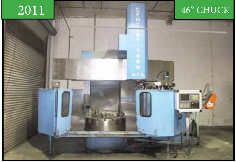
2011 (REMAN) NEW CENTURY 46" CHUCK CNC VTL W/ 12 STATION ATC, 60" SWING, FANUC OI-TD CONTROL, 4 JAW CHUCK, 6 TOOL HOLDERS, CHIP CONVEYOR, S/N :21000.
