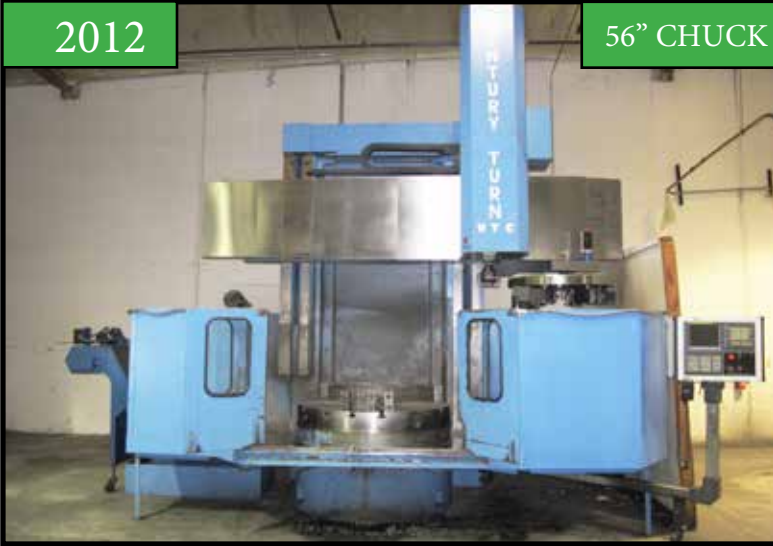
2012 (REMAN) NEW CENTURY 56" CHUCK CNC VTL W/ 12 STATION ATC, 70" SWING, FANUC OI-TD CONTROL, 4 JAW CHUCK, 6 TOOL HOLDERS, CHIP CONVEYOR, S/N:21107.
