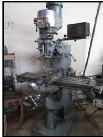
BRIDGEPORT SERIES 1 - 2HP VERTICAL MILL W/ SARGON DRO
