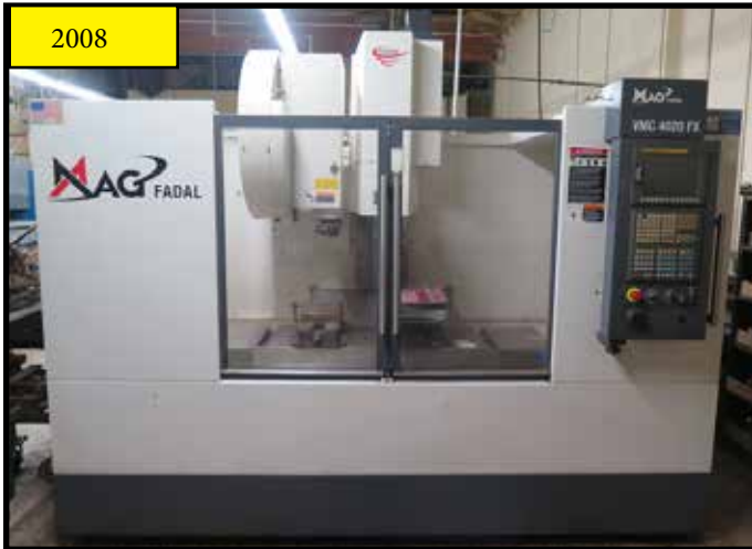
2008 MAG FADAL VMC4020FX01 CNC VERTICAL MACHINING CENTER W/ FANUC SERIES 0I-MC CONTROLS
