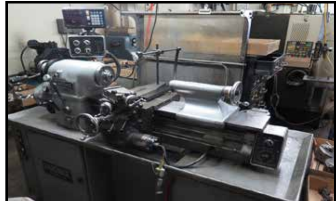
HARDINGE HLH-H WIDE BED TOOL ROOM LATHE W/ SONY DRO
