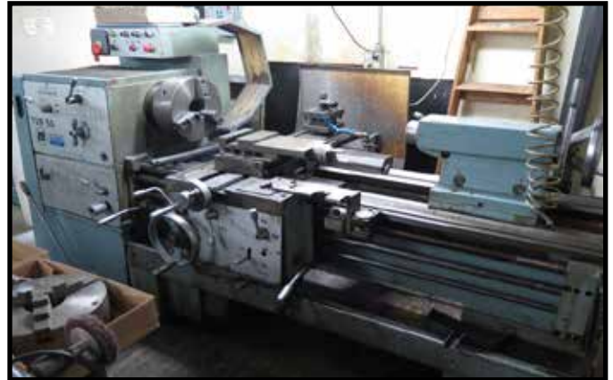
PONAR TUR-50 20" X 50" GEARED HEAD LATHE W/ 1800 RPM, 3" THRU SPINDLE BORE, TAPER ATTCH
