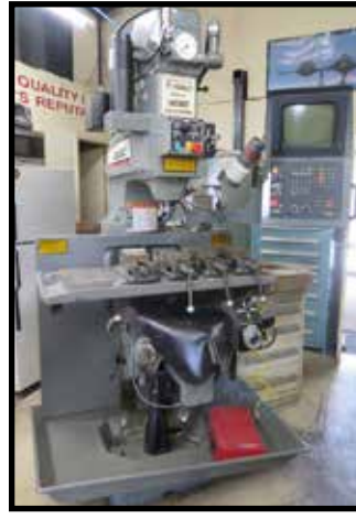
BRIDGEPORT SERIES 1 INTERACT' CNC VERTICAL MILL W/ HEIDENHAIN CON- TROLS, UNIVERSAL KWIK- SWITCH SPINDLE
