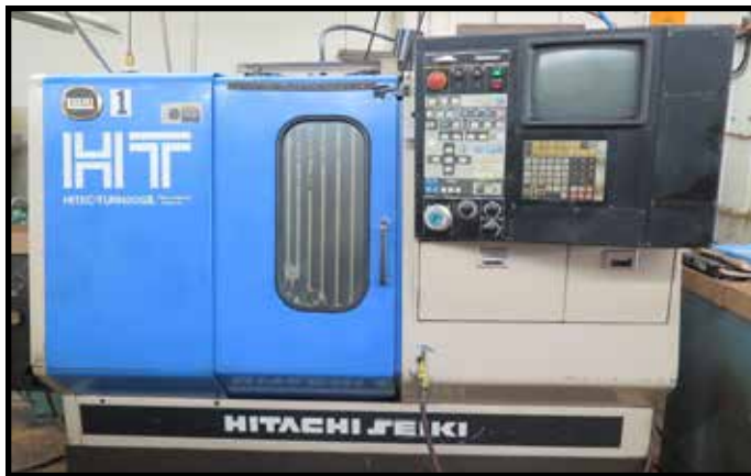
HITACHI SEIKI HITEC-TURN 20SII SUPER PRODUCTIVE TURNING CELL W/ YASNAC CONTROLS, TOOL PRESETTER
