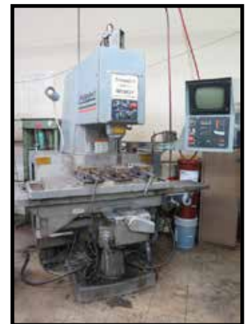
BRIDGEPORT SERIES II " " INTERACT 4" CNC VERTICAL MILL W/ HEIDENHAIN CON- TROLS, 40-TAPER SPINDLE
