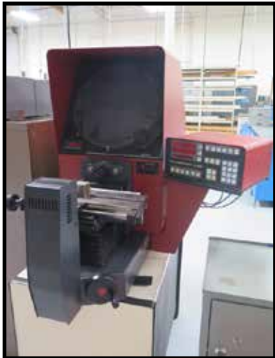
Starrett Sigma HB350 14" Optical Comparator w/ Quadra-Chek 2000 DRO
