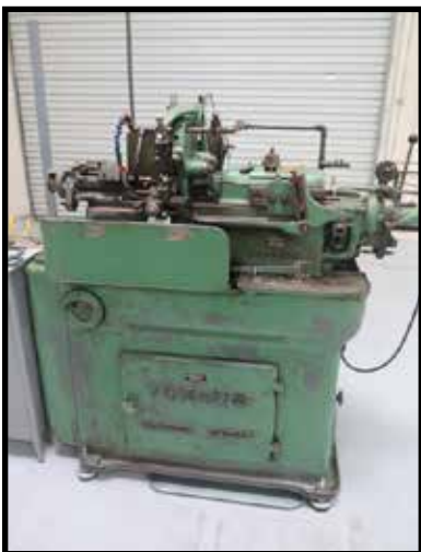
Tornos R10 10mm(.394") Cap Auto Screw Machine
