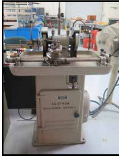
Agathon Type 150A Precision Tool Grinder w/ Diamond Wheels
