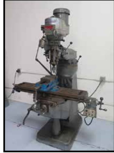
Bridgeport Series 1 - 2Hp Vertical Mill w/ 60-4200 RPM, Chrome Ways, Power Feed
