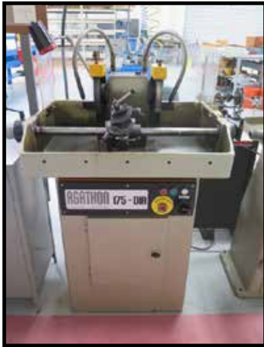
Agathon mdl. 175-DIA Precision Tool Grinder w/ Diamond Wheels
