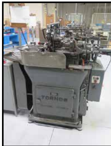
Tornos M7 7mm(.275") Cap Auto Screw Machine
