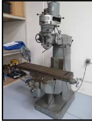
Webb S-2 Vertical Mill w/ 2Hp Motor, 80-2720 RPM, Power "Y" Feed
