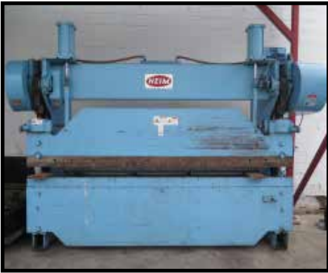
Heim mdl. 100-12 100 Ton x 12" Press Brake w/ Manual Back Gage
