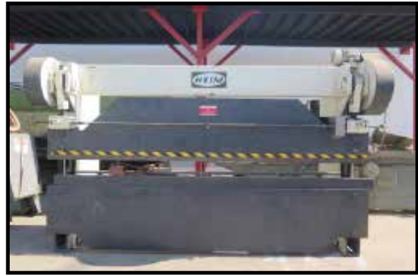
Heim 70-12 70 Ton x 12' Press Brake w/ Pneumatic Clutch
