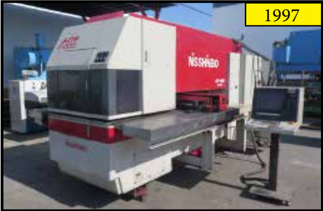
1997 Nisshinbo HTP-1000 22 Ton 22-Station CNC Turret Punch Press w/ Nisshinbo CNC Controls
