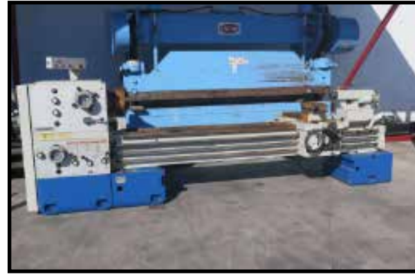
Summit 26-4X10 29" x 112" Gear-Gap Lathe w/ 4 1/8" Thru Spindle Bore
