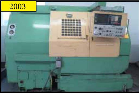
Hitachi Seiki NF-20 Twin Turret CNC Turning Center
