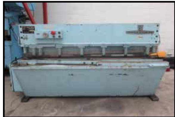
ELG "Hydra-Shear" 1/8" x 6' Deep Throat Hydraulic Power Shear
