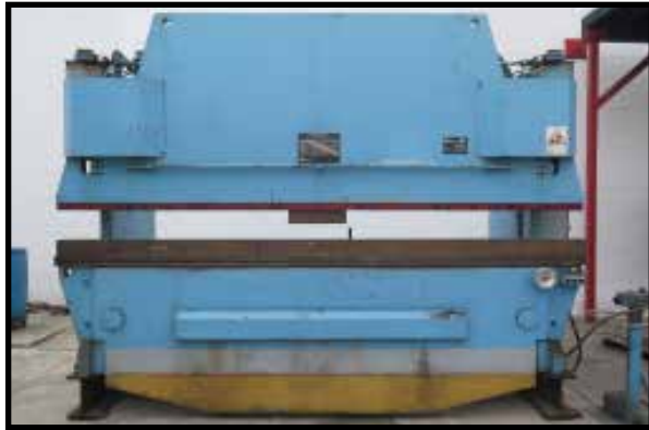
Master-Fab PC-230-12 230 Ton x 12' Hydraulic Press Brake w/ Dial Back Gage
