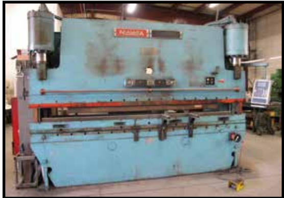
NIAGARA HBM-175-10-12, 12FT X 175 TON HYD PRESS BRAKE, W/ CYBELEC DNC 60 CONTROL, STROKE CONTROL, S/N 52275.
