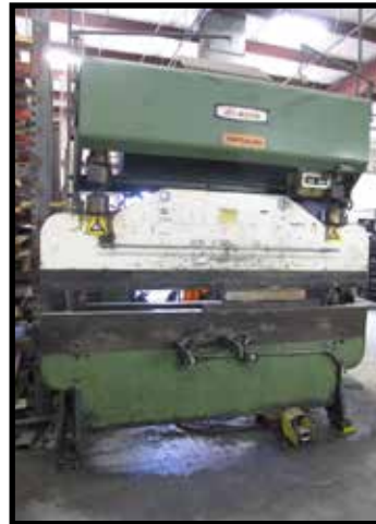
DIACRO 8FT X 55 TON HYDRO-MECHANICAL PRESS BRAKE, DUAL BUTTON CONTROL
