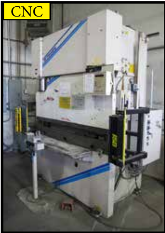
WYSONG THS100-72, 6FT X 100 TON HYD PRESS BRAKE W/ AUTO GAGE CNC BACK GAGE, ISB-PRO LIGHT CURTAINS, S/N T46-103.
