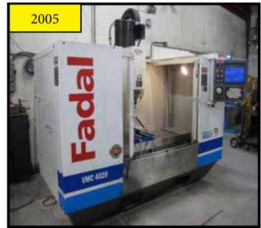
2005 2005 FADAL VMC 4020HT CNC VMC, 10,000 RPM, BT-40, 20 ATC, S/N 32005088062.
