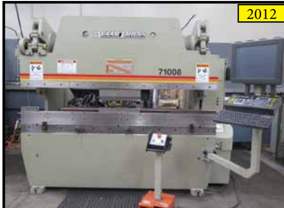
2012 Accurpress 71008 100 Ton x 8' CNC Press Brake w/ Accurpress ETS100 Controlled Gaging SYSTEM
