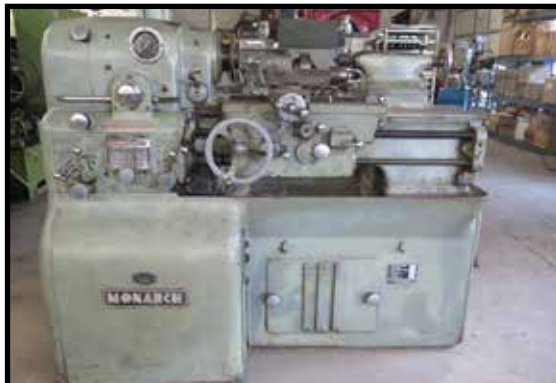
Monarch 10EE 12 1/2" x 20" Tool Room Lathe
