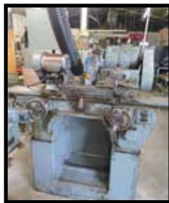
Brown & Sharpe #5 4" x 12" Auto Universal Cylindrical Grinde
