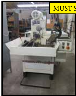
Sunnen MBC-1804 Precision Honing Machine w/ Power Stroking
