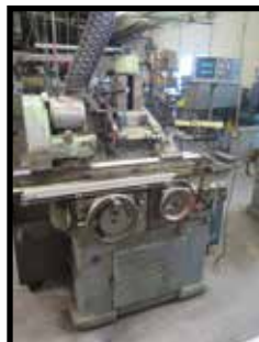
Brown & Sharpe #13 8" x 22" Universal and Tool Grinder
