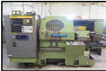
Hitachi Seiki 4NE-600 CNC Turning Center w/ Fanuc 6T Controls
