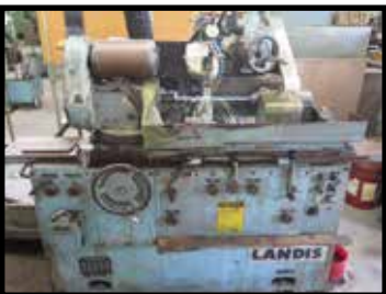
Landis Type IR 10" x 20" Universal Cylindrical Grinder
