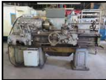
Monarch mdl. 12"-C 14 1/2" x 30" Geared Head Lathe
