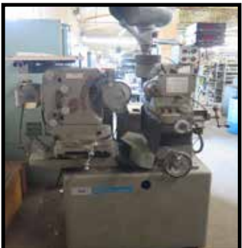
Sheffield 22VA Microform Grinder w/ Sony DRO
