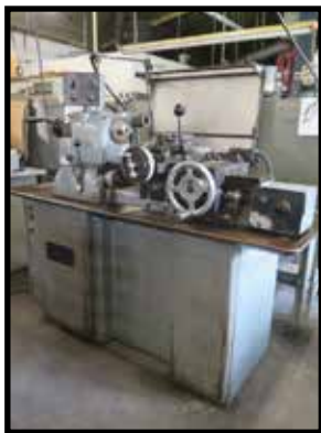
Hardinge HC Hand Chucker w/ Threading Attachment
