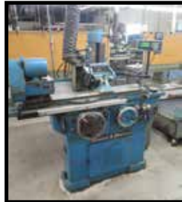
Brown & Sharpe #13 8" x 22" Universal and Tool Grinder w/ Acu-Rite DRO
