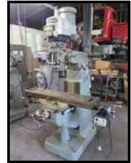
Bridgeport Vertical Mill w/ Acu-Rite DRO
