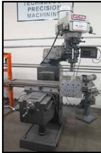
Chevalier FM-3VS Vertical Mill w/ Sony Millman DRO
