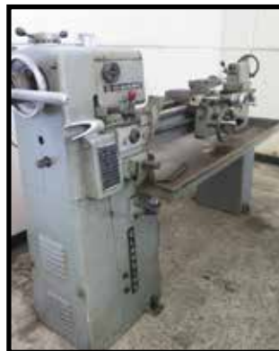
Clausing mdl. 5913 12" x 38" Lathe s/n 501040 w/ 52-2000 RPM, Inch Threading, Tailstock, 5C Collet Closer.
