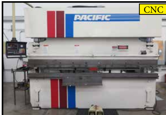
Pacific J110-10 110 Ton x 10' CNC Hydraulic Press Brake w/ Hurco Autobend 5C Controls
