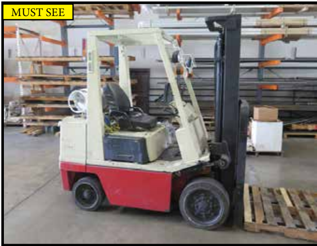
Nissan KCPH02A25PV 5000 Lb Cap LPG Forklift s/n KCPH02P904507 w/ 2-Stage Mast, 130" Lift Height, Cushion Tires, 6547 Hours.
