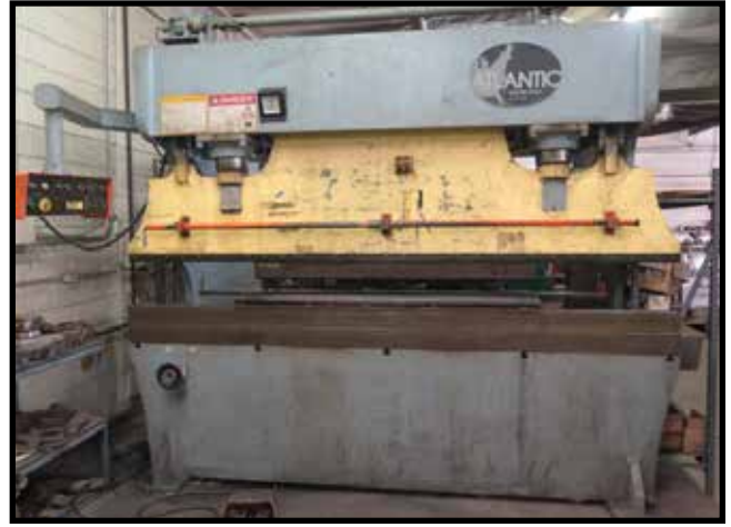
Atlantic HD200-10 200 Ton x 10' Cap Hydraulic Press Brake
