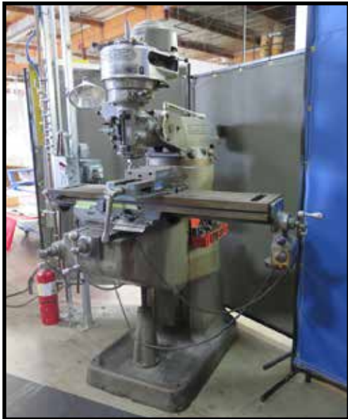
Bridgeport Vertical Mill s/n 69457 w/ 1Hp Motor, 80-2720 RPM, Power Feed, 9" x 42" Table.
