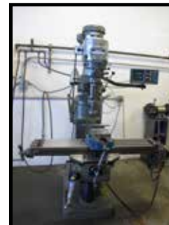
BRIDGEPORT VERT MILL WITH 2HP, DRO, P.F. TABLE, CHROME WAYS, S/N 280386
