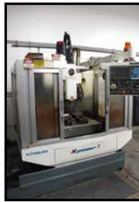
KITAMURA MYCENTER 1 CNC VMC, FANUC O-M, 10,000 RPM, 20 ATC, SIDE MOUNT TOOL CHANGER, S/N 2919.
