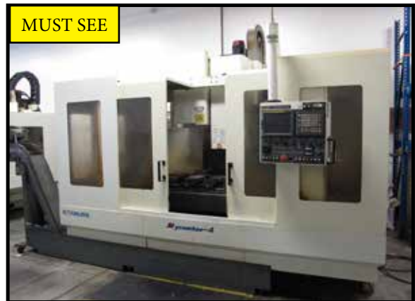
KITAMURA MYCENTER 4 CNC VMC, FANUC 16i-M CONTROL, 10,000 RPM, SIDE MOUNT TOOL CHANGER, 40 TAPER, CHIP CONVEYOR, S/N 30666.
