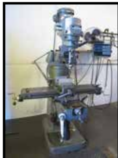
BRIDGEPORT VERT MILL WITH 2HP VAR SPEED, DRO, CHROME WAYS, S/N 264531.
