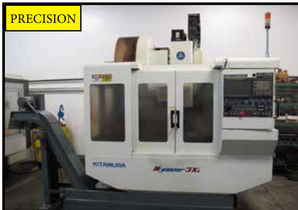
KITAMURA MYCENTER 3Xi CNC VMC, 15,000 RPM, 20 ATC, SIDE MOUNT, FANUC 16i-M CONTROL, S/N 12107.
