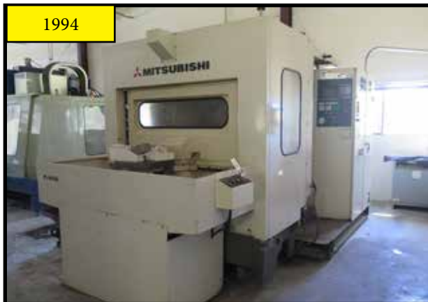
1994 Mitsubishi M-H4A 2-Pallet 4-Axis CNC Horizontal Machining Center w/ Mitsubishi Controls, 30-ATC, CAT-40 Spindle, 10,000 RPM
