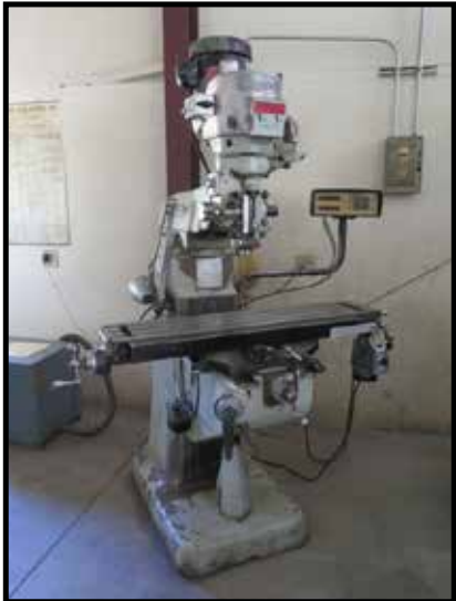
Bridgeport Series 1 - 2Hp Vertical Mill w/ Bridgeport DRO
