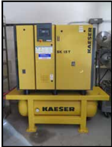
2006 Kaeser SK15T 15Hp Rotary Air Compressor
