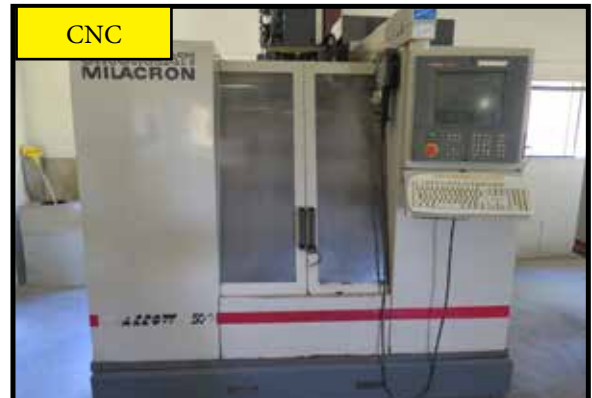
Cincinnati "Arrow 500" CNC Vertical Machining Center w/ Acramatic 2100 Controls
