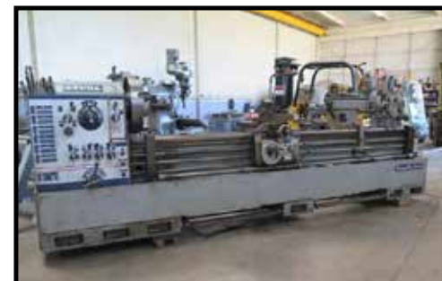
Tuda TudorMax 23X118 Geared Head Gap Bed Lathe s/n 20013 w/ 3 1/8" Thru Spindle Bore, 21-1500 RPM, Inch/mm Threading, Tailstock.
