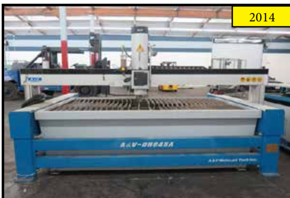
2014 A&V 5' x 8' Cap CNC Waterjet 410,MPa Max Pressure S/N: 1405-001
