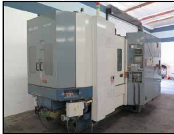
Mori Seki SH-50 2-Pallet CNC HMC, w/Fanuc MSC-516 MB, CAT 40, 40 ATC S/N: 606
