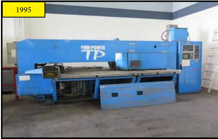
1995 Finn-Power mdl. TP2525 IF2/21/AM CNC Turret Punch Press w/ Sinumerik System 3 Controls, 21-Station Turret
