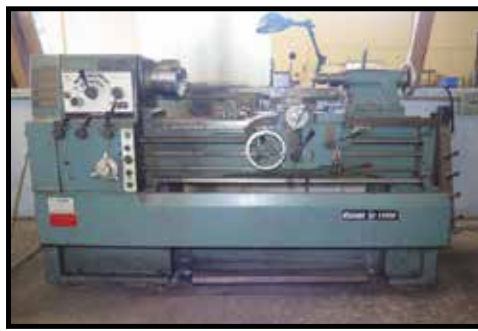
Poncho / Osama Sr. 1740G 17" x 40" Geared Head Gap Bed Lathe s/n 202011 w/ 32-2000 RPM, Inch Threading, Tailstock.
