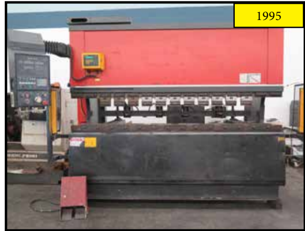
1995 AMADA FBD-1030E, 100 Ton x 10' CNC Press Brake w/ 3 Axis NC9-EXII Control
