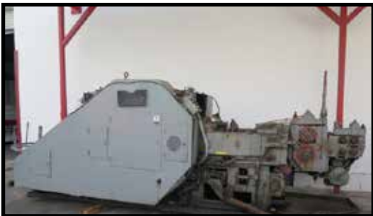
National Machinery 1/2" Cold Nut Former / Cold Header
