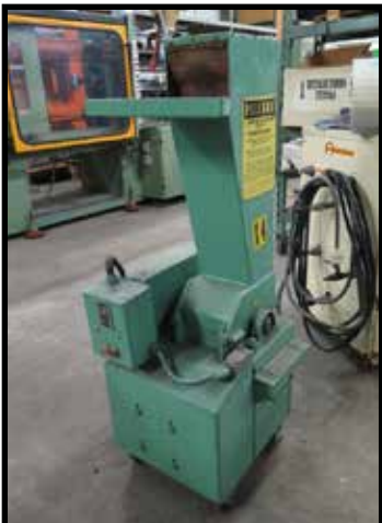
Flinchbaugh 6" Plastics Granulator
