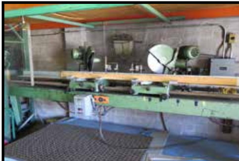
STB Dual Head Miter Saw w/ Power Feeds
