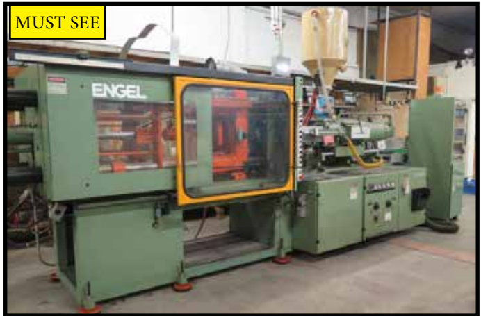
Engel ES700/175 175 Ton Plastic Injection Molding Machine
