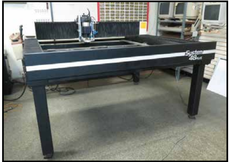
Gerber SYSTEM-48 PLUS 5' x 6' CNC Router
