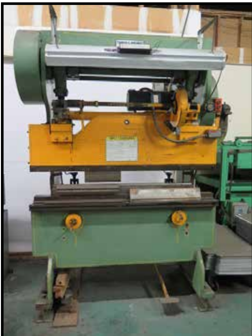
Chicago 60'' Press Brake w/ Back Gage, Motorized Slide Adj
