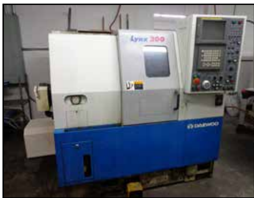
2001 Daewoo LYNX200 CNC Turning Center w/ Fanuc Series 21i-T Controls, Tool Presetter, 12-Station Turret, 6000 Max Spindle RPM, Rigid Tapping
