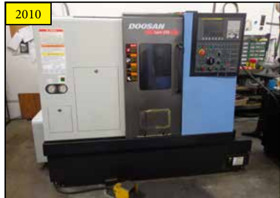
2010 2010 Doosan LYNX220A CNC Turning Center w/ Doosan-Fanuc i-Series Controls, 12-Station Turret, 6000 Max Spindle RPM, Hydraulic Tailstock, Rigid Tapping
