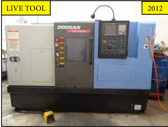
2012 2012 Doosan LYNX220 LMA CNC Live Turret Turning Center w/ Doosan-Fanuc i-Series Controls, Tool Presetter, 12-Station Live Turret, 6000 Max Spindle RPM, 6000 Live Turret RPM, Full "C" Axis, Hydraulic Tailstock, 2" Thru Spindle Bore, Rigid Tapping
