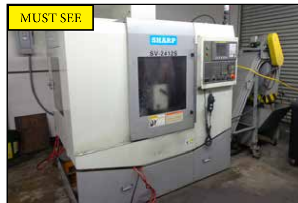
2009 Sharp SV-2412S 4-Axis CNC Vertical Machining Center w/ Fanuc Series 0i-MC Controls, 16-Station ATC, CAT-40 Spindle 10,000 RPM, Rigid Tapping, ATS/Rockwell 4th Axis Rotary
