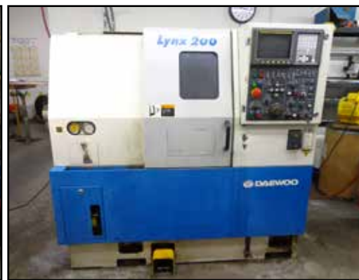
1998 Daewoo LYNX200 CNC Turning Center w/ Fanuc Series 21-T Controls, 12-Station Turret, 6000 Max Spindle RPM, Hydraulic Tailstock
