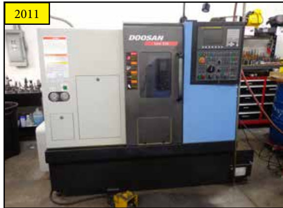
2011 2011 Doosan LYNX220A CNC Turning Center s/n ML0013-0005275 w/ Doosan-Fanuc i-Series Controls, Tool Presetter, 12-Station Turret, 6000 Max Spindle RPM, Hydraulic Tailstock
