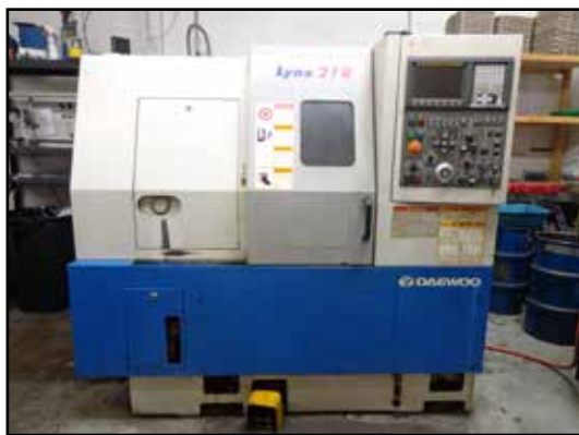
2003 Daewoo LYNX210A CNC Turning Center w/Daewoo-Fanuc i-Series Controls, 12-Station Turret, 6000 Max Spindle RPM, 1 3/4" Thru Spindle Bore
